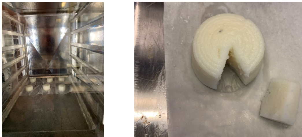
Figure 2.3.6. Example of steam cooking in lab testing to imitate typical water bath cooking of surimi in industry (left). Cooked and gelled surimi product, pH shift paste after 5 days of storage (right).
