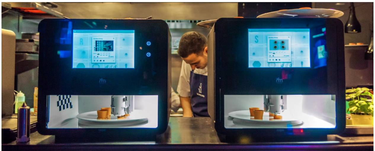
Figure 1.1.2. A pair of Foodini 3D printers from Natural Machines, which extrude food from a system of refillable capsules, meaning you're free to print with practically any ingredients you choose (Photo: Natural Machines).
