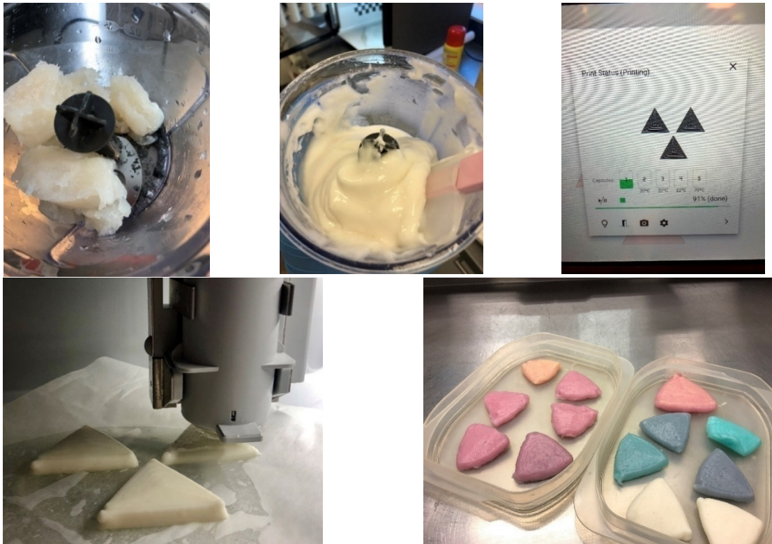
Figure 2.4.7.1. Schematic of process. Cooked surimi paste product (orange colored triangles (1.5 mm nozzle) mixed with astaxanthin omega 3-fatty acid oil). The grayish purple hue triangles are made with Icelandic volcanic salt.
