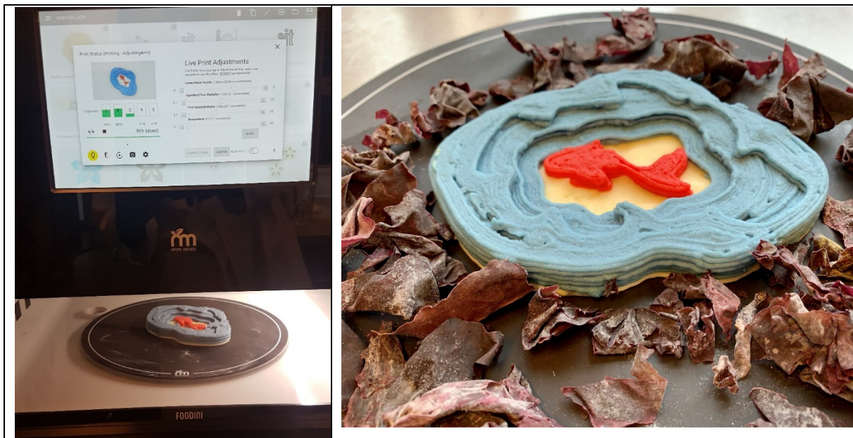
Figure 3.2.3. „Fish in water“ shape printed in Foodini 3D printer. Three capsules are needed, fish ingredients and other ingredients with different colors can be utilized (left). „Fish in water“ shape with dulce showcased (right).
