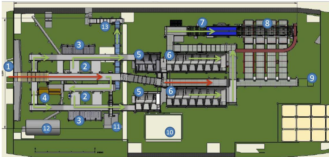
FIGURE 2 PROCESSING LAYOUT ONBOARD GROUND FISH TRAWLER (1. RECEPTION UNIT - 2. BLEEDING/GUTTING/SORTING STATION - 3. COLLECTION BOXES FOR BY-CATCHES - 4. GUTTING MACHINE - 5. BLEEDING IN FRESH SEAWATER - 6. PRE-COOLING IN RSW- 7. MEASURING & MONITORING - 8. SORTING - 9. HATCH DOWN TO HOLD - 10. ACCESS PANEL TO THE HOLD FOR LANDING THE CATCHES - 11. STORAGE FOR LIVER AND ROE - 12. RSW RESERVOIR TANK 13. DISCARD CHUTE.
