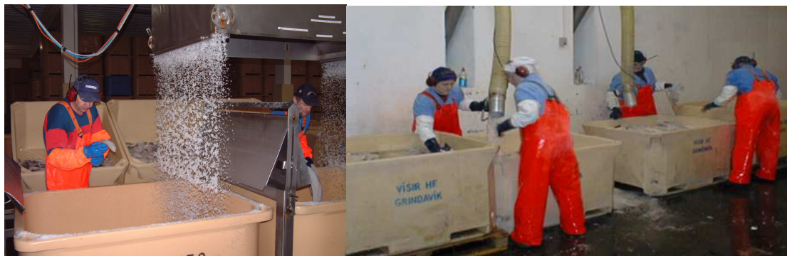
FIGURE 16 DRY SALTING AND BRINE SALTING
