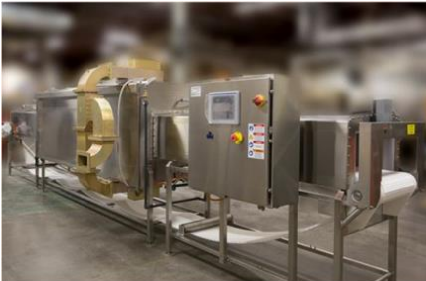
Figure 10: Ferrite's continuous industrial tempering unit
