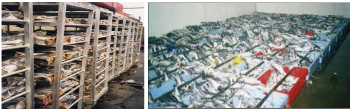
Figure 2: Thawing in still air. Fish is placed on special racks that stand on the factory floor
