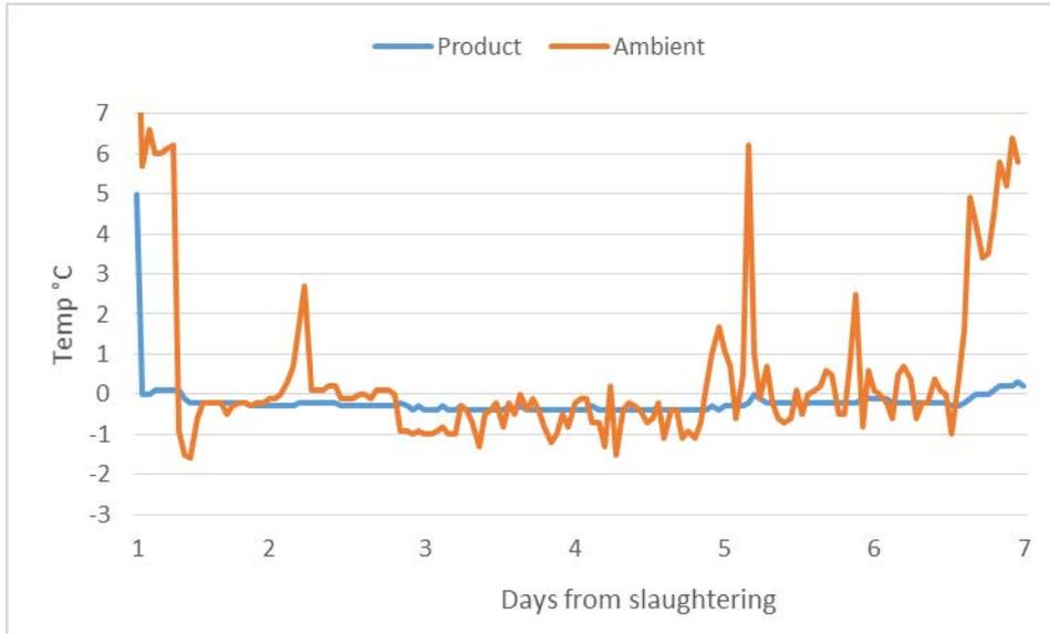
**Figure 28 Temperature profile within the product as well of the ambient condition during transportation from Norway to Italy.**
