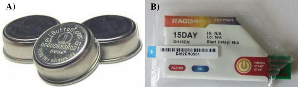
**Figure 3. A) IButton DS1922L temperature loggers used to monitor the temperature within the product and the ambient temperature. B) TempSEN ITAG-PRO PDF single use temperature logger used to monitor the temperature of product and the ambient temperature.**
