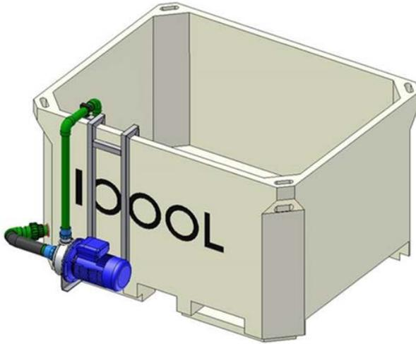
**Figure 1** Schematic figure of the sub-chilling tub equipped with a centrifugal pump to recycle the chilled brine.
