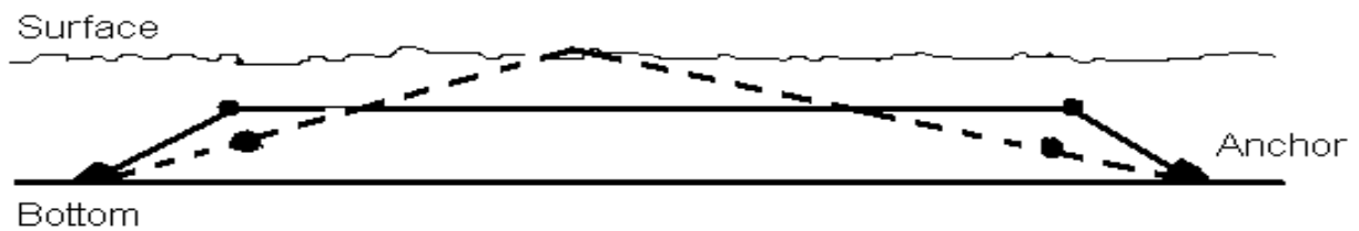
Figure 4. Long-line with drag-anchors
