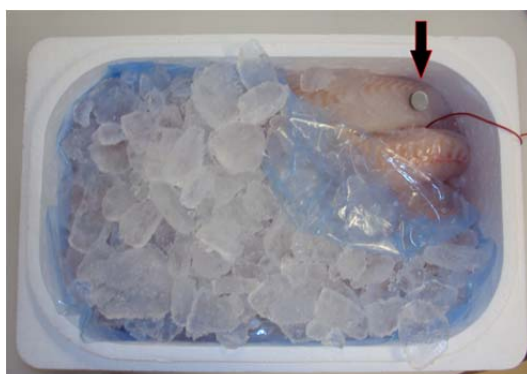
Figure 4. Whole haddock fillets in an EPS box. Also shown are temperature loggers used for monitoring temperature on top of fillets.
