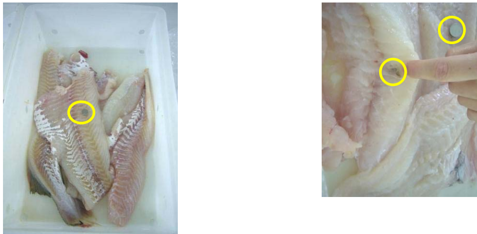
Figure 26. Fillets placed in a plastic box on a plastic table simulating the waiting period during breaks in trimming (left) and position of temperature recorder inside the fillet (right). The temperature recorders are marked with yellow circles.
