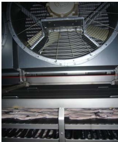
Figure 16. Inside a CBC cooler, fillets are laid down on the skin and cooled with blast and contact cooling.
