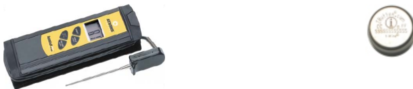
Figure 7. AccuTuff Plus 330 digital thermocouple thermometer (left) and iButton DS1922L temperature recorder (right).
