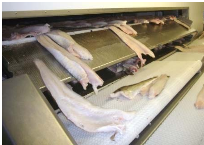
Figure 17. Fillets exiting a CBC cooler, the fillets are laid on a conveyor belt which transports them to skinning and trimming. Fillet temperature is around -1 to -0.5\text{ }^\circ\text{C} after CBCC.
