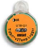
Figure 3. The Onset temperature data loggers
