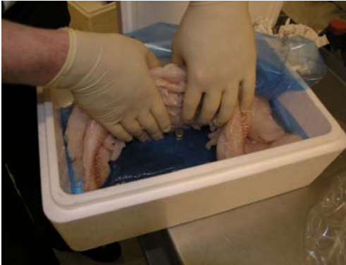
Figure 33. DS1922L ibutton logger at the bottom centre of an EPS box.
