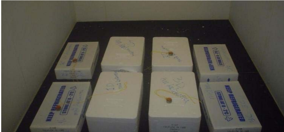
Figure 14. Four EPS boxes and four CP boxes placed on the floor of Chamber 1-2.
