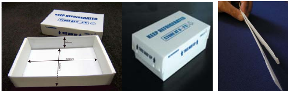
Figure 6. Corrugated plastic box (CP, brand: Coolseal). Left: whole box. Right: cut through the box walls.
