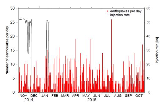
Figure 11. KJ-39 injection rate and earthquake activity.
