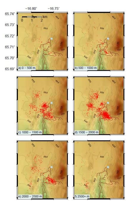
**Figure 5.** Seismic activity distribution in different depth intervals. Each figure a) – e) represents a 500 m thick layer. Figure f) shows all events located deeper than 2500 m. The main activity occurs between 1000 and 2000 m depth where the activity is clearly divided into 5 different clusters.
