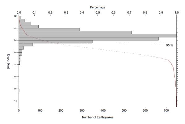
**Figure 4.** Depth distribution of the events located in Krafla area. The main activity occurs in 1000 to 2250 m depth. 95 % of the earthquakes are located shallower then 2225 m.
