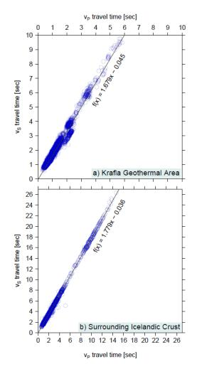
**Figure 8.** Vp/Vs ratio in Krafla geothermal area and the surrounding crust. In Krafla the Vp/Vs ratio has been calculated to 1.679, outside the area it appears to be 1.779 what is consistent with other studies on the Icelandic crust (e.g. Brandsdóttir and Menke, 2008; Tryggvason et al. 2001) where values are typically around 1.75 to 1.79.
