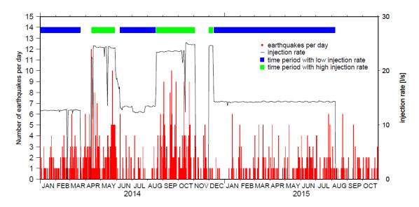
**Figure 12.** *IDDP-1* borehole injection rate and seismic activity. Blue bars mark time periods of low injection rate that are used for analysis and green bars marks those with high injection rate.
