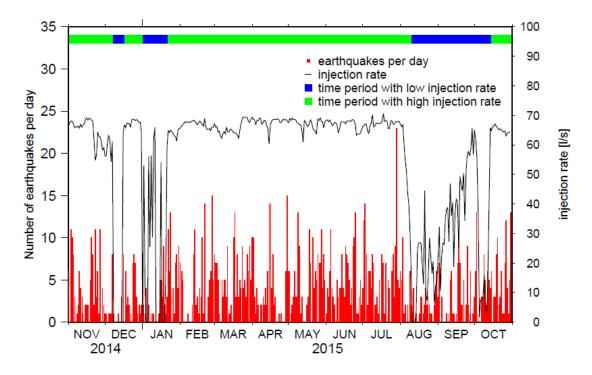
**Figure 10.** KG-26 injection rate and earthquake injection. Time periods marks green are considered to be times with high injection rate. The blue marked times with low or irregular injection rate.
