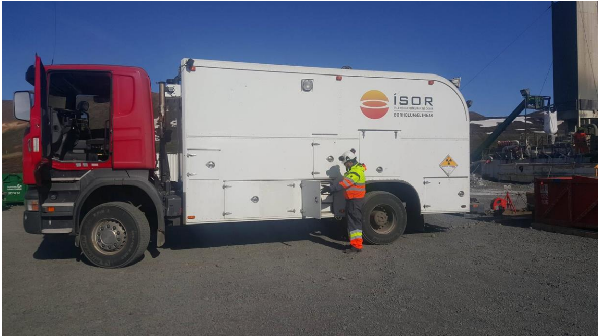
Figure 1. ÍSOR's logging engineers preparing for geophysical logging in well bG-11.
