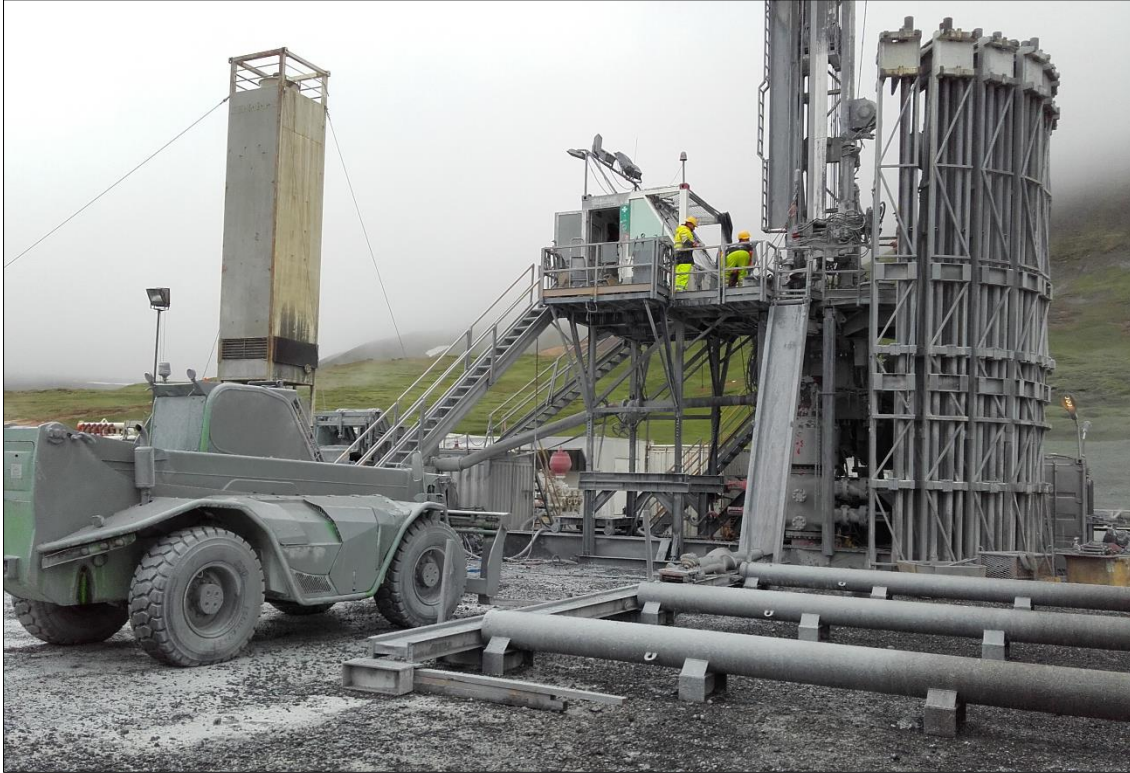
Figure 10. Mud and debris at well pad A after a blow-out from PG-10 at 5:45 am on July 3 rd .
