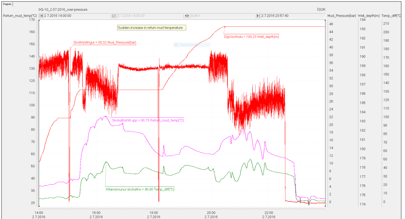
Figure 11. Increased return mud temperature (pink curve) at 3:30 pm on the 2 nd of July.
