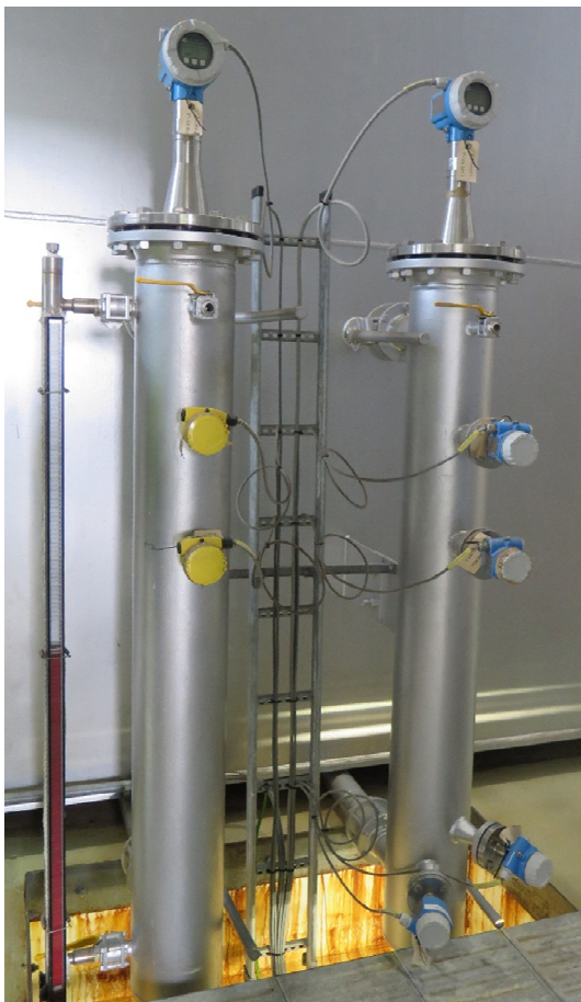
FIGURE 27: Radar and Vegaswing sensors for water level control
