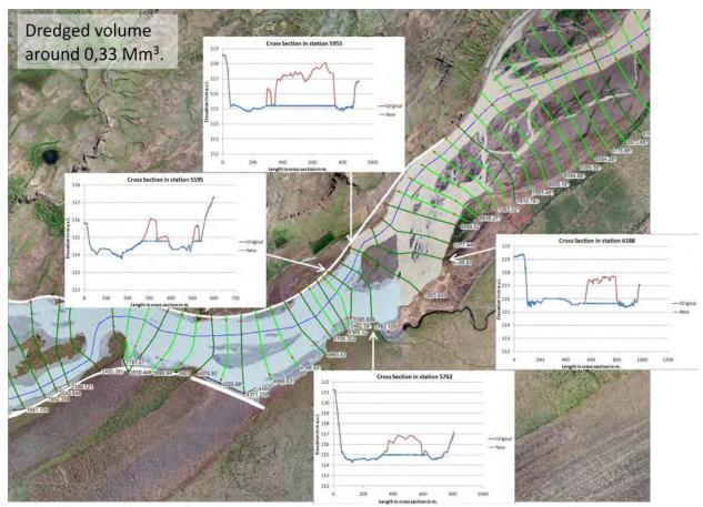
**Figure A4.5** *The bathymetry of the river is changed by removing the reef.*
