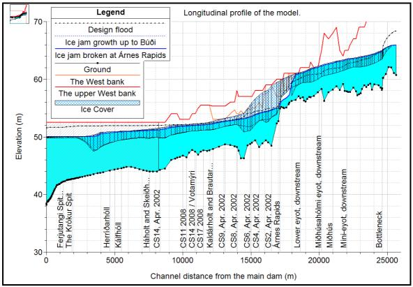
**Figure 7.14** *The West Bank of the river with the longitudinal profile of two freeze-up ice jams and the design flood as a comparison.*
