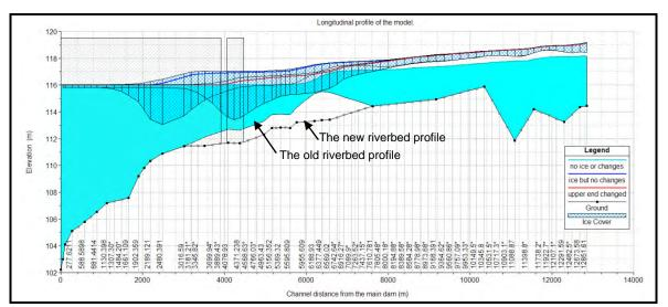
**Figure A4.10** The changed longitudinal profile is the red one. Above the junctions there are no changes so only the lower part of the model is shown.
