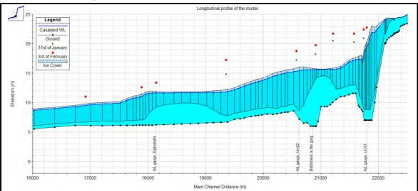
**Figure A2.3** Test using  $n_i$  = dense slush,  $\phi = 25^{\circ}-30^{\circ}$  and  $p_j = 0,5$  in order to calibrate the model to the extremes in 2004.
