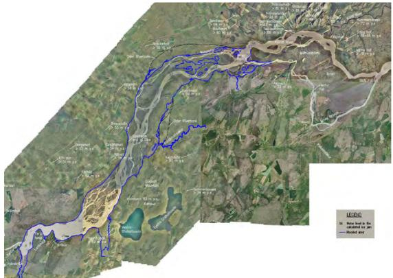
**Figure 7.11** Overview of how high the water can rise due to a continuous wide river ice jam reaching all the way up to the shallows below Árnes Rapids. Discharge 300  $m^3/s$ . An A3 version of this figure can be found at the end of this report before the Appendixes.
