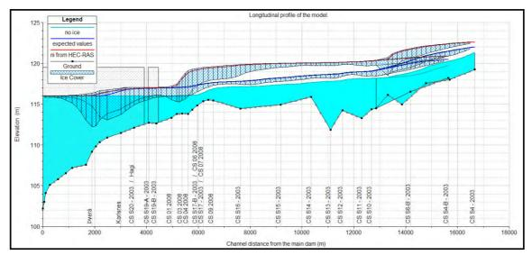
**Figure 6.12** The longitudinal profile of the Hagalón Ice Jam where  $n_i$  has been calculated in HEC-RAS, i.e. using the Nezhikhovskiy's relationship for ice floes.
