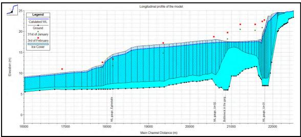
**Figure A2.4** Test using  $n_i = 0,12$ ,  $\phi = 20^\circ$  and  $p_j = 0,6$  in order to calibrate the model to the extremes in 2004.
