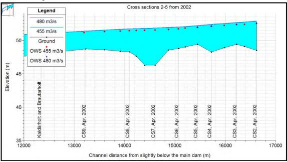
Figure 7.6 Calibration of cross sections 2-5 from 2002. OWS stands for observed water surface.
