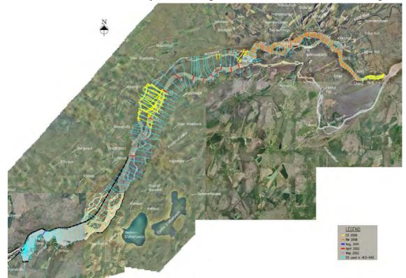
**Figure 7.1** An overview of both measured cross sections (CS) in the model area and the location of the cross sections used in the Heiðarlón model. An A3 version of this figure can be found at the end of this report before the Appendixes.
