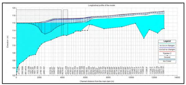
**Figure A4.4** *The changed longitudinal profile is the red one. Very small changes. Above the junctions there are no changes so only the lower part of the model is shown.*
