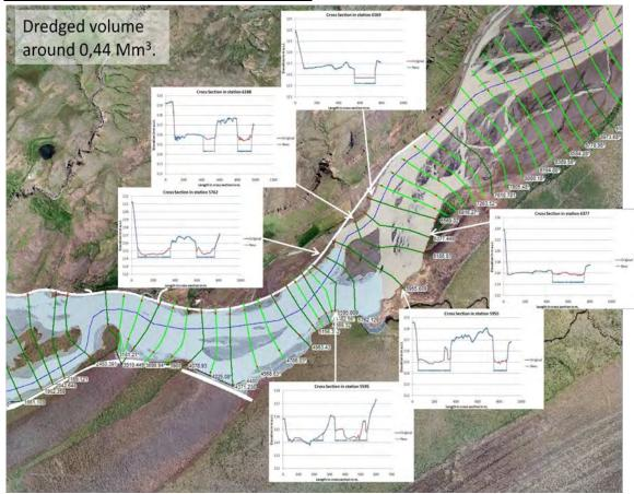
**Figure A4.7** *The bathymetry of the river is changed by removing the shallows.*
