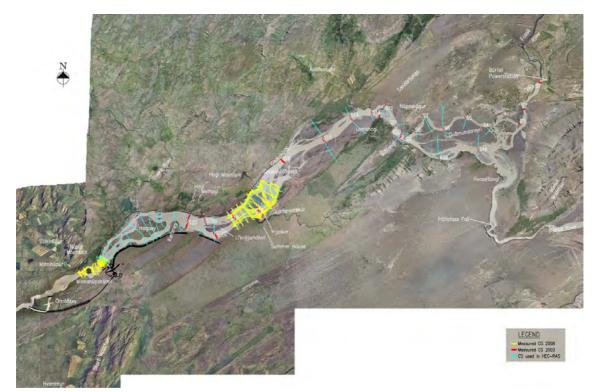
**Figure 6.1** An overview of both measured cross sections (CS) in the model area and the location of the cross sections used in the Hagalón model. An A3 version of this figure can be found at the end of this report before the Appendixes.
