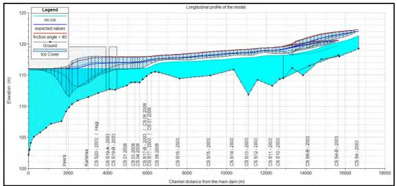
Figure 6.11 The longitudinal profile of the Hagalón Ice Jam where  $\phi$  has been lowered to 40°.
