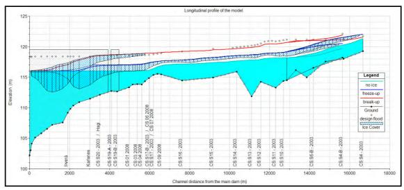
**Figure 6.15** *The same as above, but with the internal friction angle for the break-up ice jam changed to 50.*
