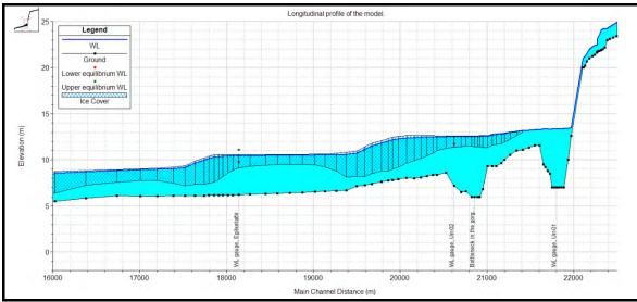
Figure A2.13 Calibration of the early stages of Urriðafoss Ice Jam.
