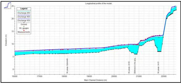
Figure A2.2 Calibration of the reach without ice.
