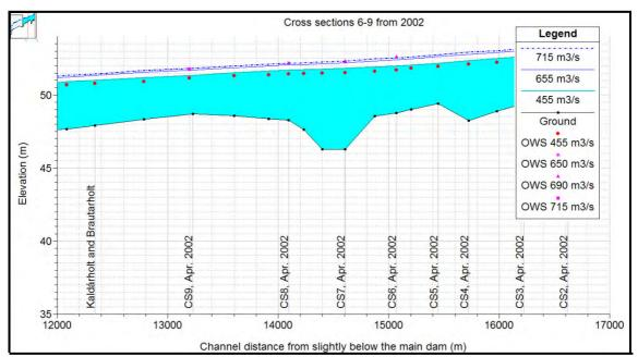
Figure 7.5 Calibration of cross sections 6-9 from 2002. OWS stands for observed water surface.
