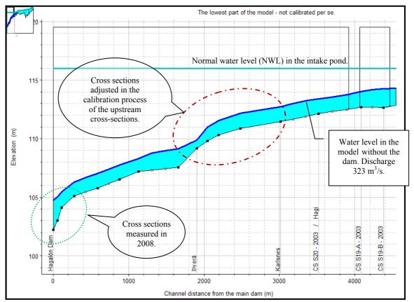
Figure 6.3 Longitudinal profile of the Hagalón Pond.
