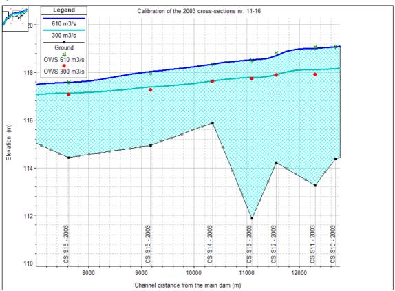
Figure 6.5 Calibration of cross sections nr. 11-16, from November 2003.
