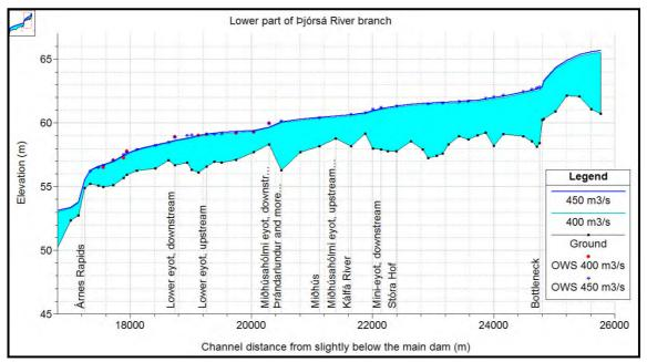
**Figure 7.8** Calibration of the lower part of the reach from Árnes Rapids up to Búði Fall. OWS stands for observed water surface.
