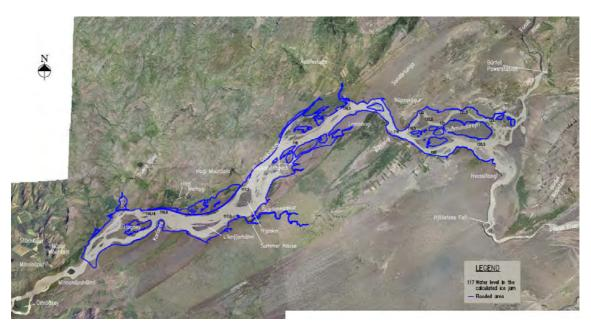
**Figure 6.10** Overview of how high the water can rise due to a continuous wide river ice jam reaching all the way up to the roots of Búrfell Mountain. Discharge 300  $m^3$ /s. An A3 version of this figure can be found at the end of this report before the Appendixes.
