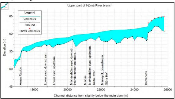
Figure 7.9 Calibration of the reach from the bottleneck up to Búði Fall. OWS stands for observed water surface.
