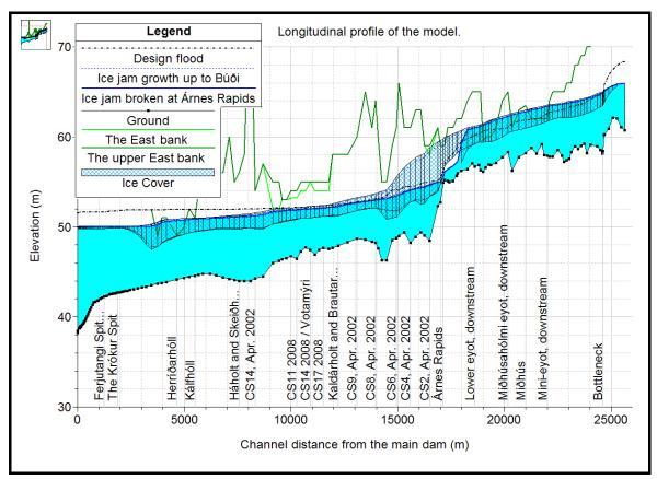
**Figure 7.15** *The East Bank of the river with the longitudinal profile of two freeze-up ice jams and the design flood as a comparison.*
