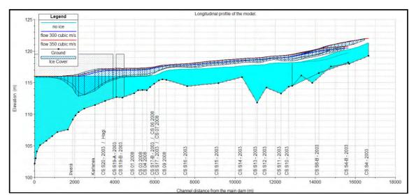
**Figure 6.13** *The longitudinal profile of the Hagalón Ice Jam where the flow has been changed from 300*  $m^3$ /*s to 350*  $m^3$ /*s. Expected values used for ice variables.*
