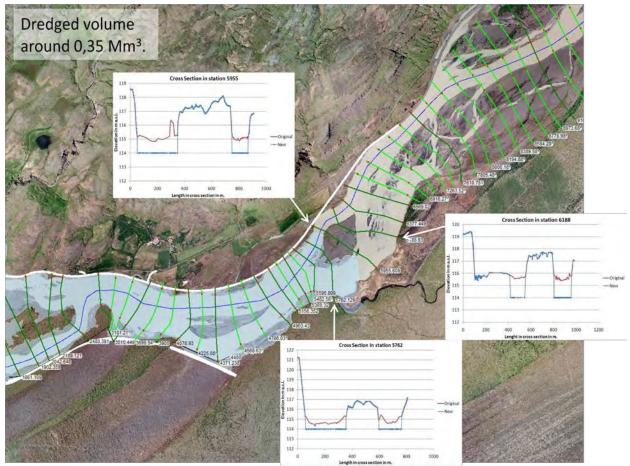
**Figure A4.1** The bathymetry of the river on either side of the reef is lowered down to 114 *m a.s.l. in three cross-sections.*
