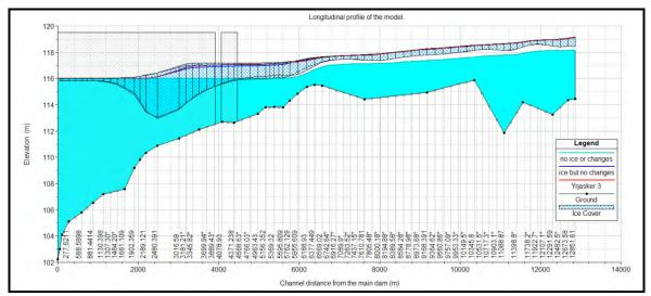
**Figure A4.6** *The changed longitudinal profile is the red one. Very small changes. Above the junctions there are no changes so only the lower part of the model is shown.*
