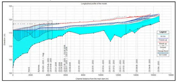
**Figure 6.14** The longitudinal profile of a possible break-up ice jam with expected values, a discharge of  $1500 \text{ m}^3$ /s and same ice mass as the freeze-up ice jam. Water level for no ice and expected freeze-up ice jam for discharge of  $300 \text{ m}^3$ /s and the design flood for the hydroelectric project is also shown.
