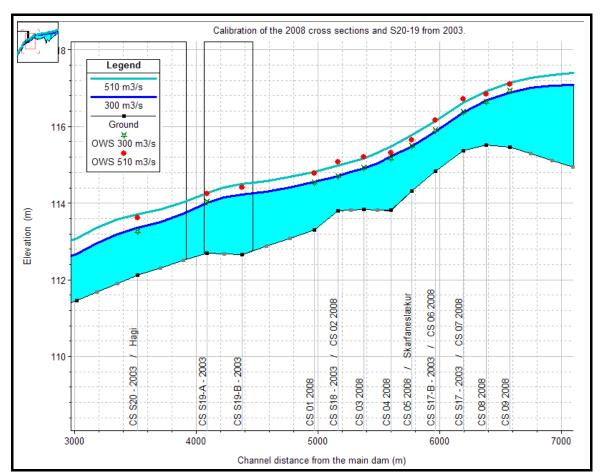
Figure 6.4 Calibration of the cross sections taken in the summer of 2008 and cross sections 19 & 20 from 2003.
