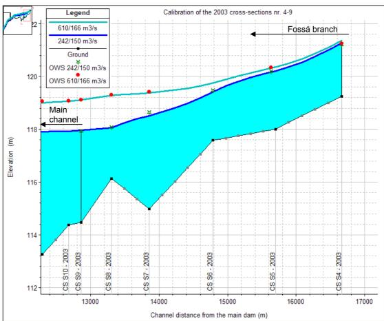
Figure 6.7 Calibration of cross-sections nr. 4-9, from November 2003.
