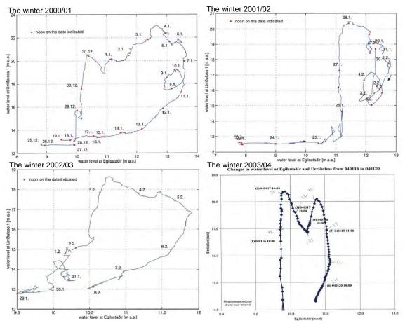
**Figure A2.12** Copies of graphs from two reports by Gunnar and Victor (2003 & 2006). Showing the relationship between the waterlevel at Egilsstaðir gauge and Urriðafoss 01 gauge. Based on this the early phases of the formation of the Urriðafoss Ice Jam was calibrated. Figure A2.13 shows the final result. It was found by using
