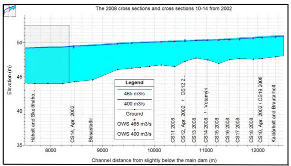
**Figure 7.4** Calibration of the cross sections from 2008 and cross sections 10-14 from 2002. The shaded area is the dike and OWS stands for observed water surface.
