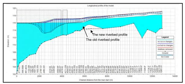
**Figure A4.8** The changed longitudinal profile is the red one. Again small changes. Above the junctions there are no changes so only the lower part of the model is shown.
