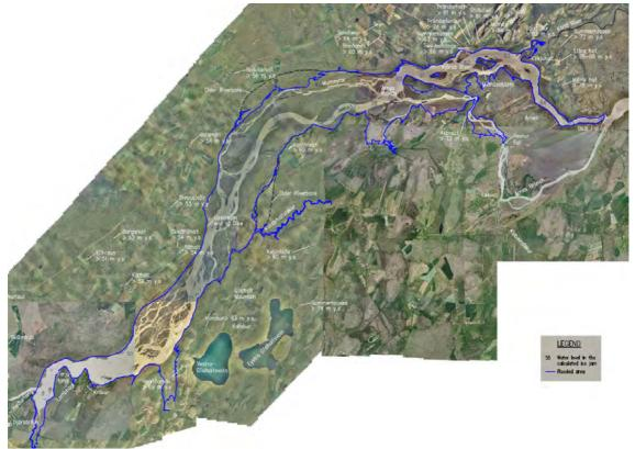
**Figure 7.13** Overview of how high the water can rise due to a continuous wide river ice jam reaching all the way up to the pond below Búði Fall. Discharge  $300 \text{ m}^3$ /s. An A3 version of this figure can be found at the end of this report before the Appendixes.
