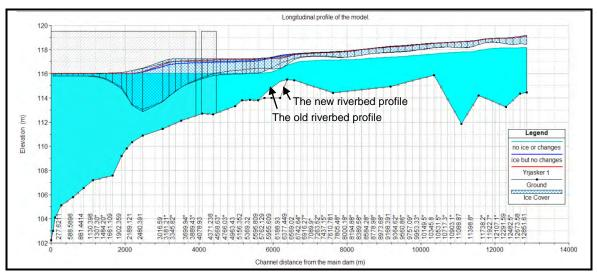
**Figure A4.2** *The changed longitudinal profile is the red one. Very small changes. Above the junctions there are no changes so only the lower part of the model is shown.*
