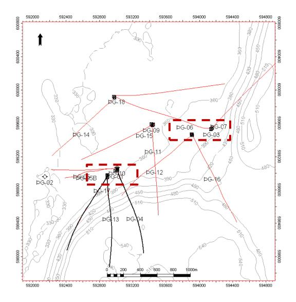
**Figure 12.** Location of well pad A and well pad C, where over-pressurized feed zones were cut. The over pressure was also recognized in well PG-9 but did not cause any problem during drilling.
