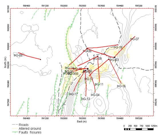
**Figure 1.** Location of the Deistareykir production wells, surface manifestations, surface faults and fissures and roads in the area.
