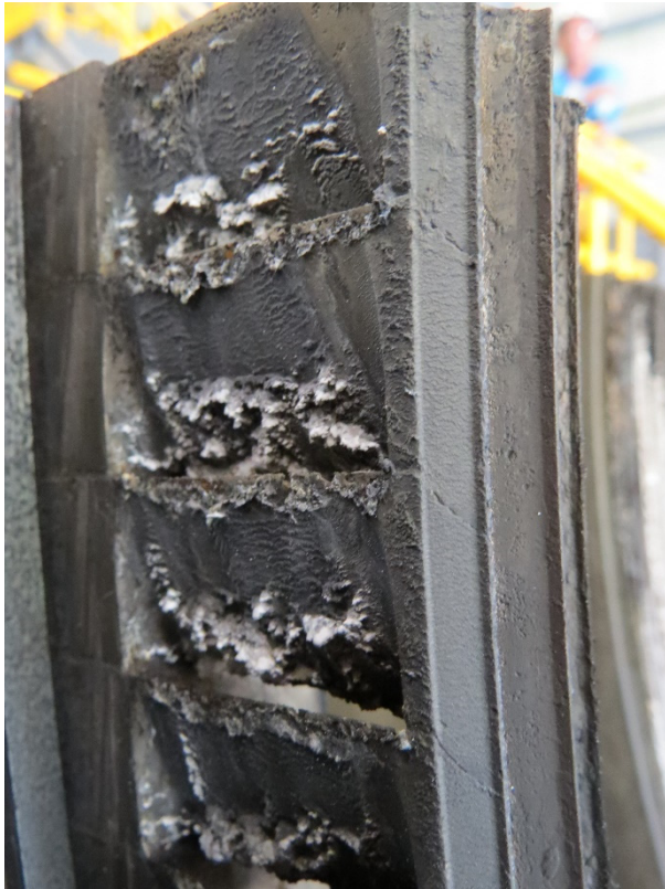
FIGURE 13: Close up view of the 1 st stage upper stationary blades (trailing edge)
