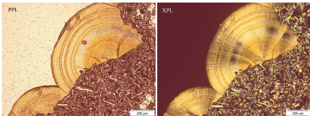
FIGURE 6: Spherical radiating siderite precipitated on fine-grained basalt at 226 m
