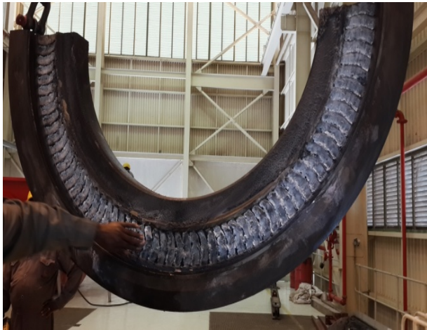
FIGURE 2: Clogged turbine nozzles
