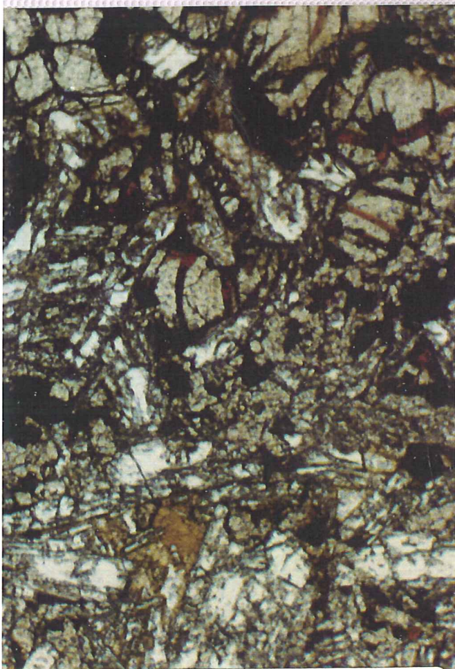
Photo no 6.5 FV-10 Depth 34.7 m thin section no 15278 Olivine basalt
