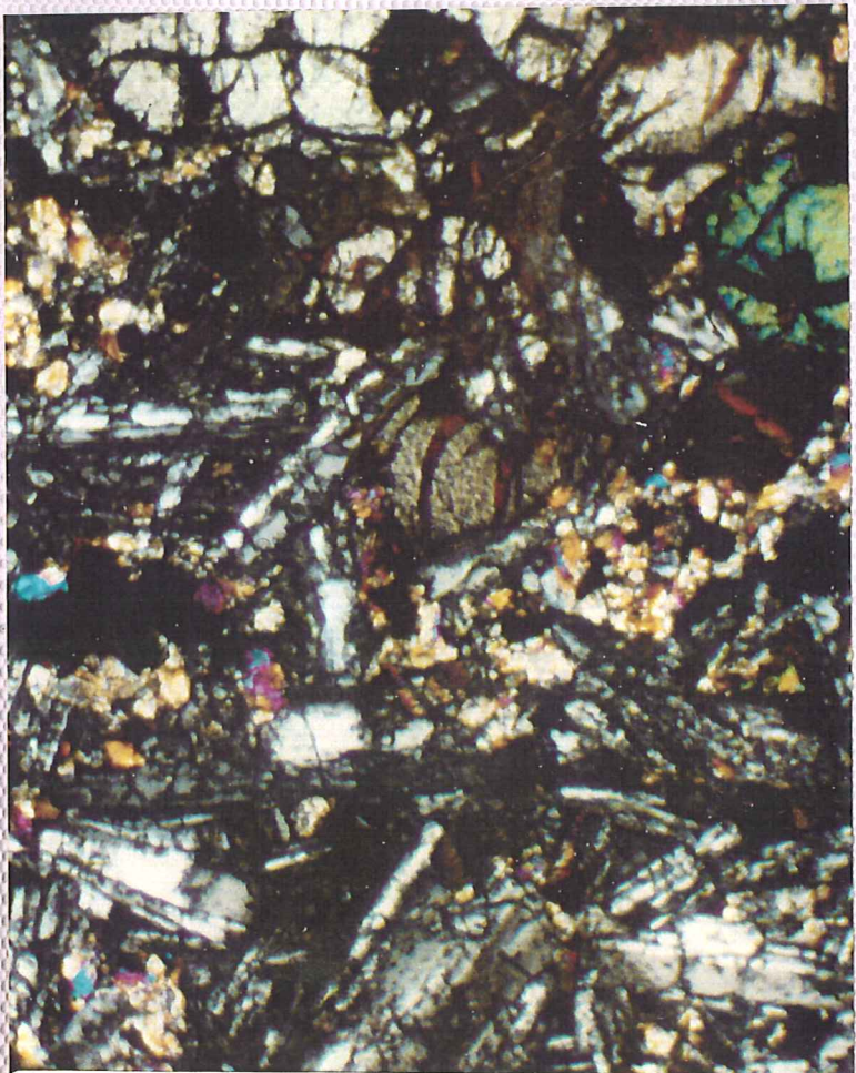
Photo no 6.6 FV-10 Depth 34.7 m thin section no 15278 Olivine basalt
