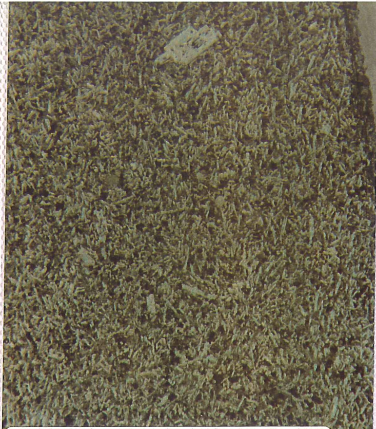
Photo no 6.8 FV-8 Depth 136.2 m thin section no 15277 Porphyritic basalt
