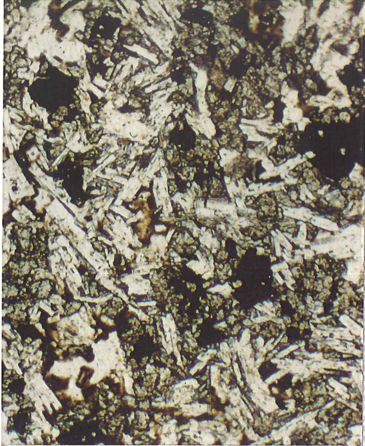
Photo no 6.1 FV-1 Depth 465.2 m thin section no 15276 Tholeiitic basalt
