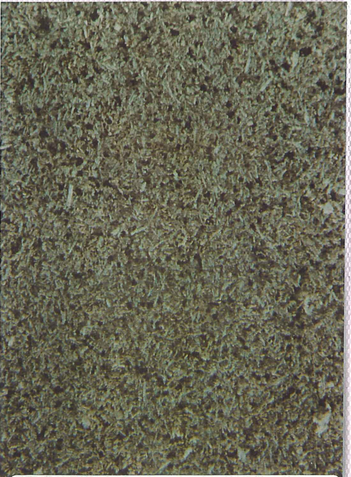
Photo no 6.7 FV-1 Depth 465.2 m thin section no 15276 Tholeiitic basalt
