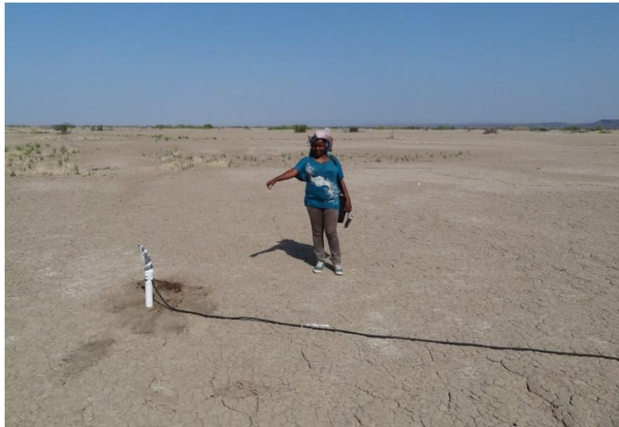
FIGURE 27: Burying the vertical magnetic sensor
