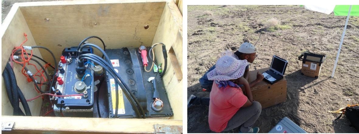
FIGURE 28: Left: Connected data logger; Right: Checking the online status of data acquisition
