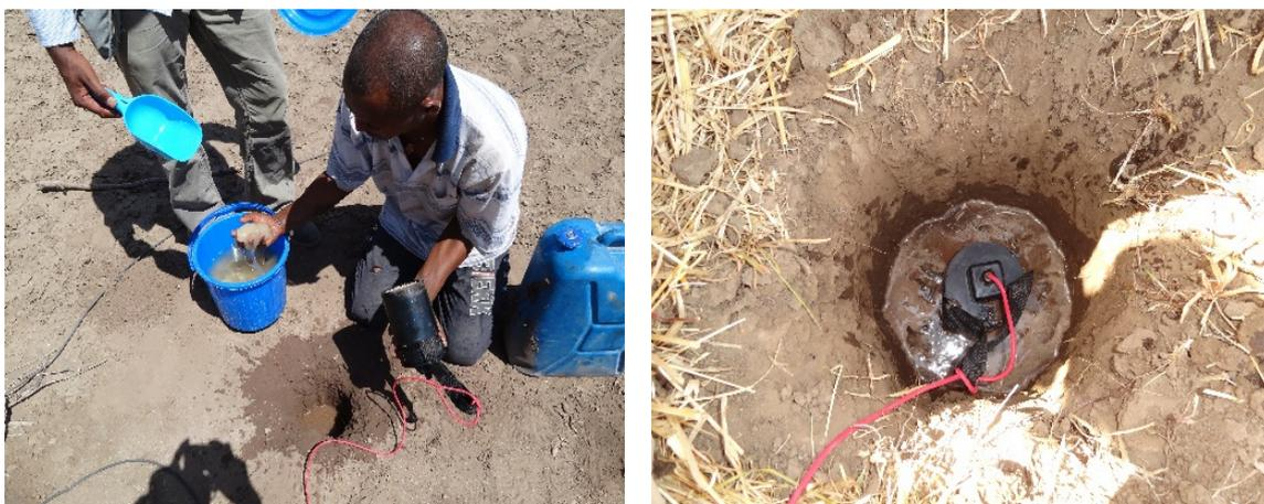
FIGURE 25: Right: Hole filled with a mixture of salty water, bentonite and soil; Left: Electrode installed in a hole 40 cm deep and ready to be covered with soil
