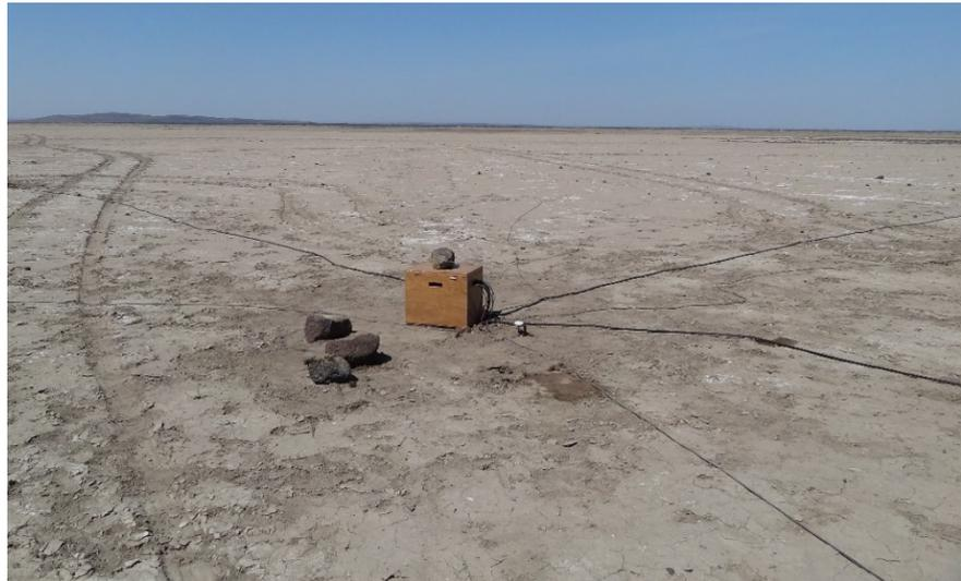
FIGURE 29: Wooden box used for protecting the data logger from the sun and wind
