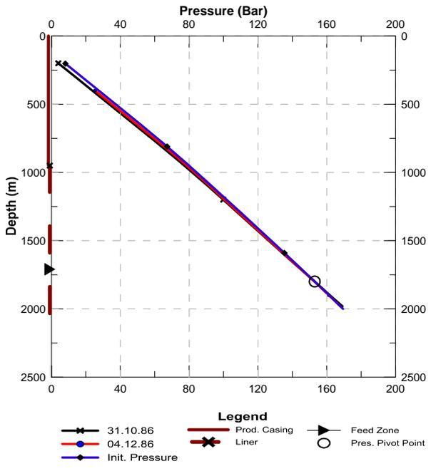
FIGURE 24: Pressure profiles for well NJ-18
