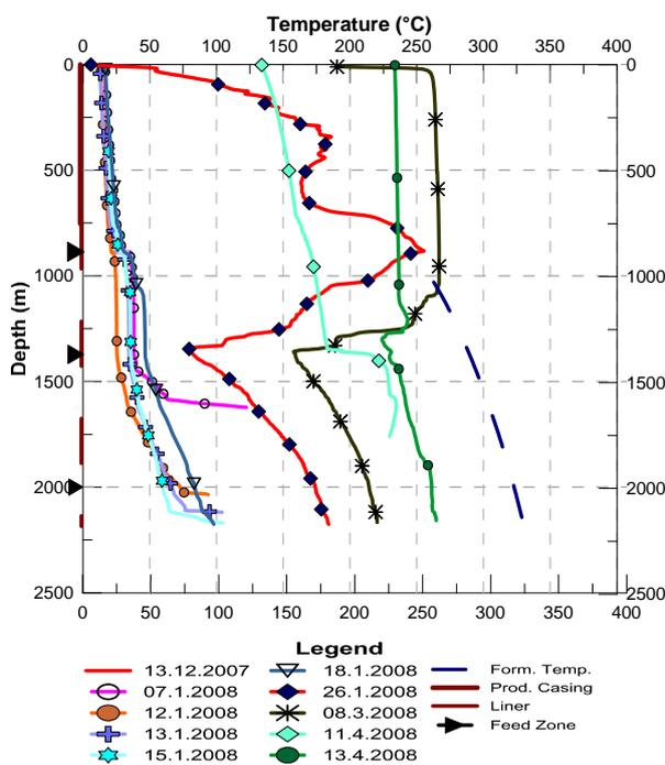
FIGURE 27: Temperature profiles for well K-37
