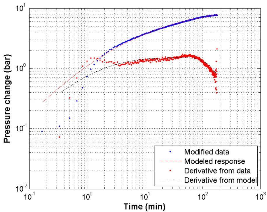
FIGURE 19: Pressure and its derivative against time for model results and collected data for step 3 on a log-log scale
