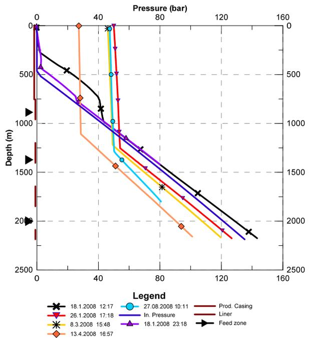
FIGURE 28: Pressure profiles for well K-37
