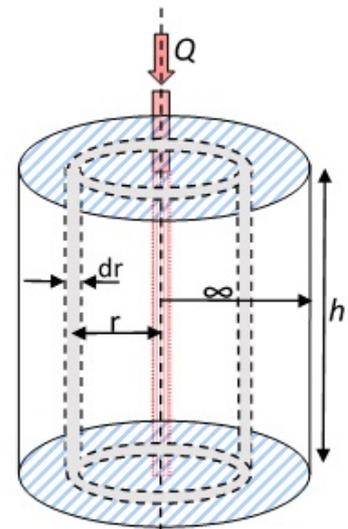
FIGURE 3: Radial flow through a cylindrical shell
