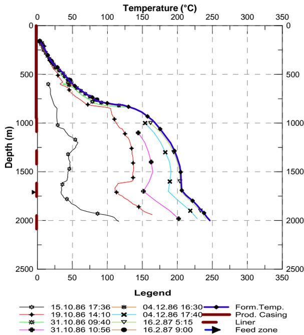
FIGURE 23: Temperature profiles for NJ-18
