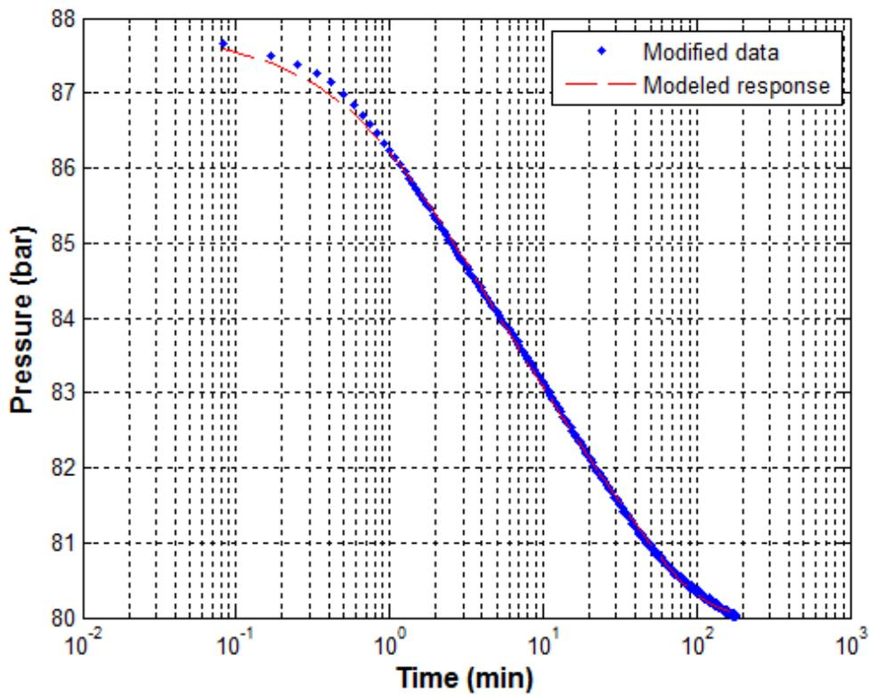
FIGURE 14: Pressure against time for model results and collected data for step 3, using a logarithmic time scale
