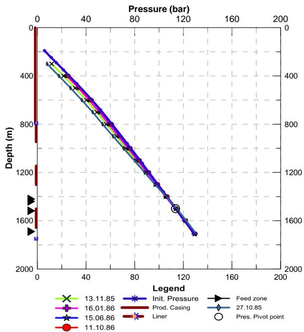
FIGURE 22: Pressure profiles for well NJ-15
