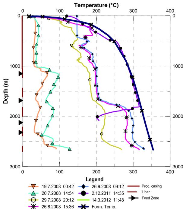
FIGURE 25: Temperature profiles for well K-38
