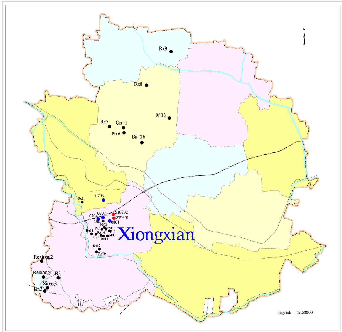
FIGURE 4: Distribution of geothermal wells in Xiongxian; injection well ST0902, production well ST0901 and observation wells 0307, 0703, 0704 and 0801 are shown
