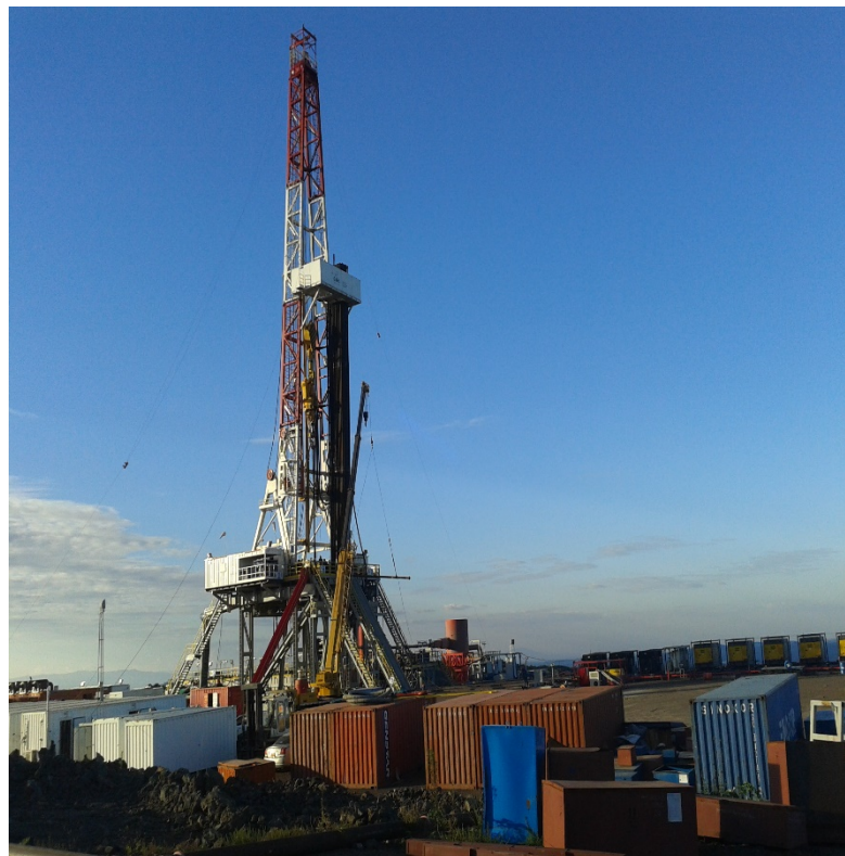
FIGURE 5: Rotary drill rig
