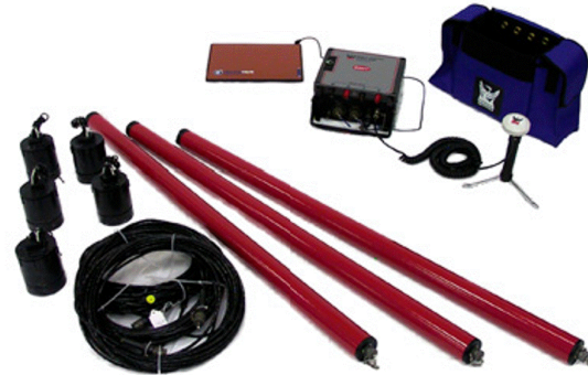
FIGURE 32: Phoenix V5-2000 MT system. From left to right; five non-polarizing electrodes, 3 induction coil cables, 3 MTC-50 induction coils, battery, MTU-5 recording unit, GPS antenna, and case for the unit. The picture is taken from Phoenix Geophysics website
