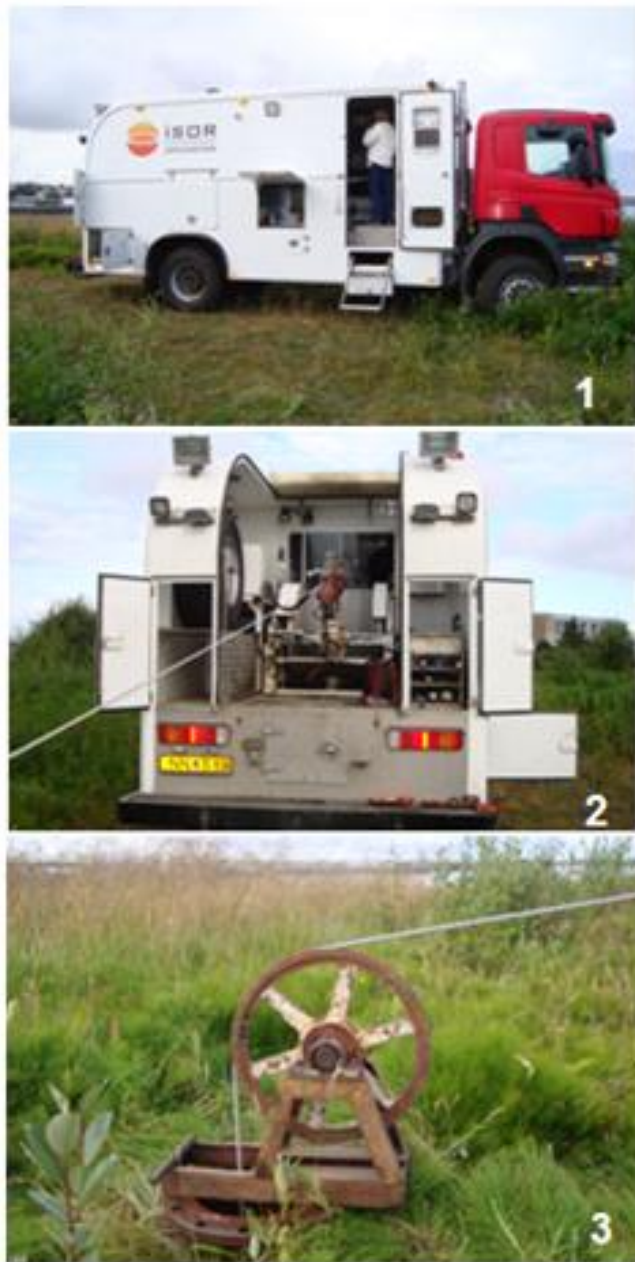
FIGURE 6: Data acquisition system; 1) Logging truck; 2) Logging equipment; 3) Well HS-36
