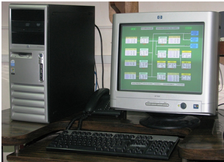
FIGURE 4: Master Terminal Unit – MTU located at the CSRG
