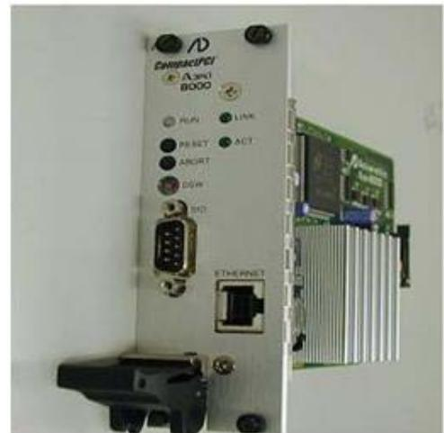
FIGURE 17: CPCPU01 Compact PCI CPU card
