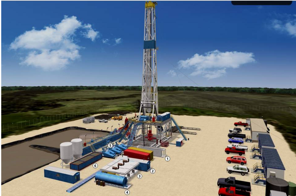
FIGURE 3: View 2 of a drilling platform and main components (J. Perez Graphics & Design, 2007): 1. SCR house/ top drive; 2. SCR house/ generator; 3. Engine / generator set; 4. Fuel tank; 5. Mud pumps; 6. Water tank
