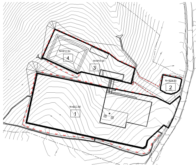
FIGURE 17: View of levels and survey of the Chinameca drill site; 1. Main terrace; 2. Parking; 3. Sludge tank and drying area; and 4. Water tank terrace
