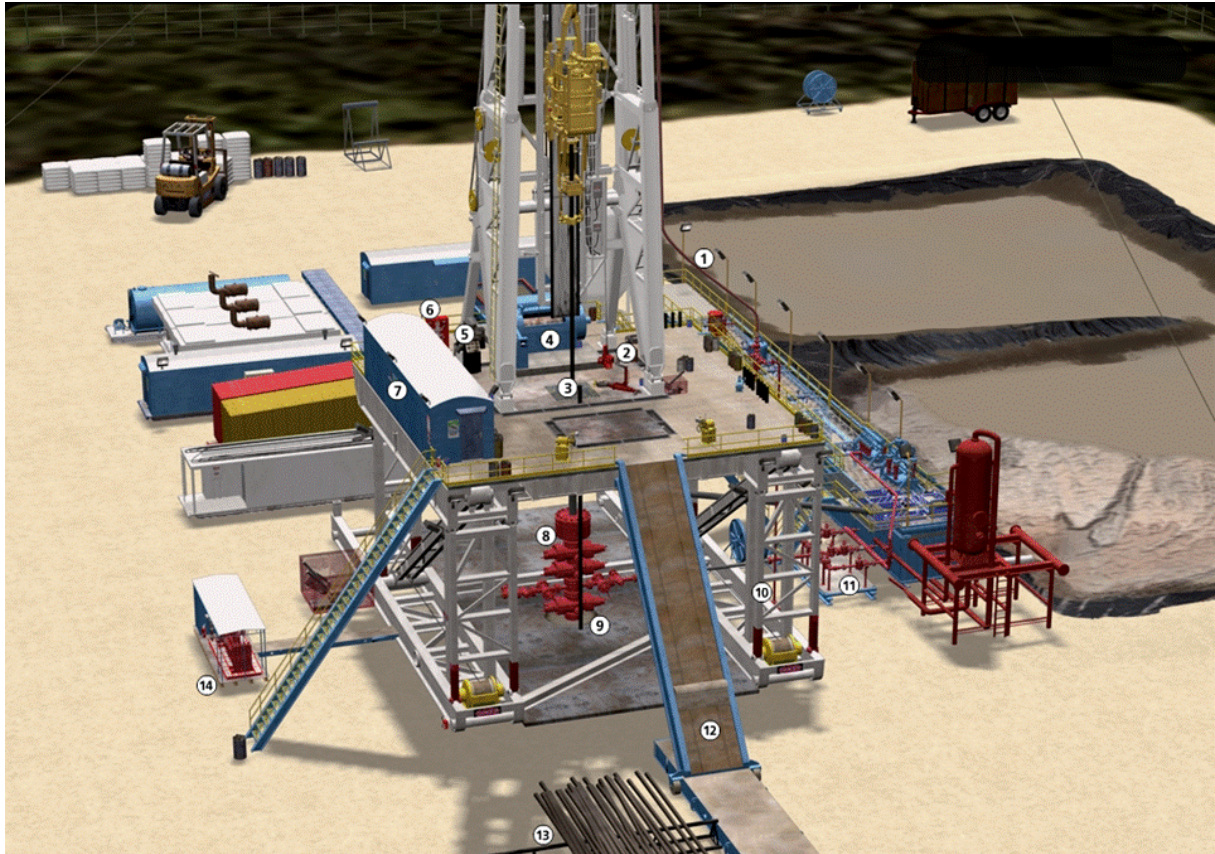
FIGURE 4: View 3 of a drilling platform and main components (J. Perez Graphics & Design, 2007): 1. Stand pipe, 2. Iron roughneck, 3. Rotary Table, 4. Draw works, 5. Driller's console, 6. BOP controller, 7. Dog house, 8. BOP stack, 9. Cellar, 10. Substructure, 11. Choke manifold, 12. Cat walk, 13. Pipe rack, 14. Accumulator.
