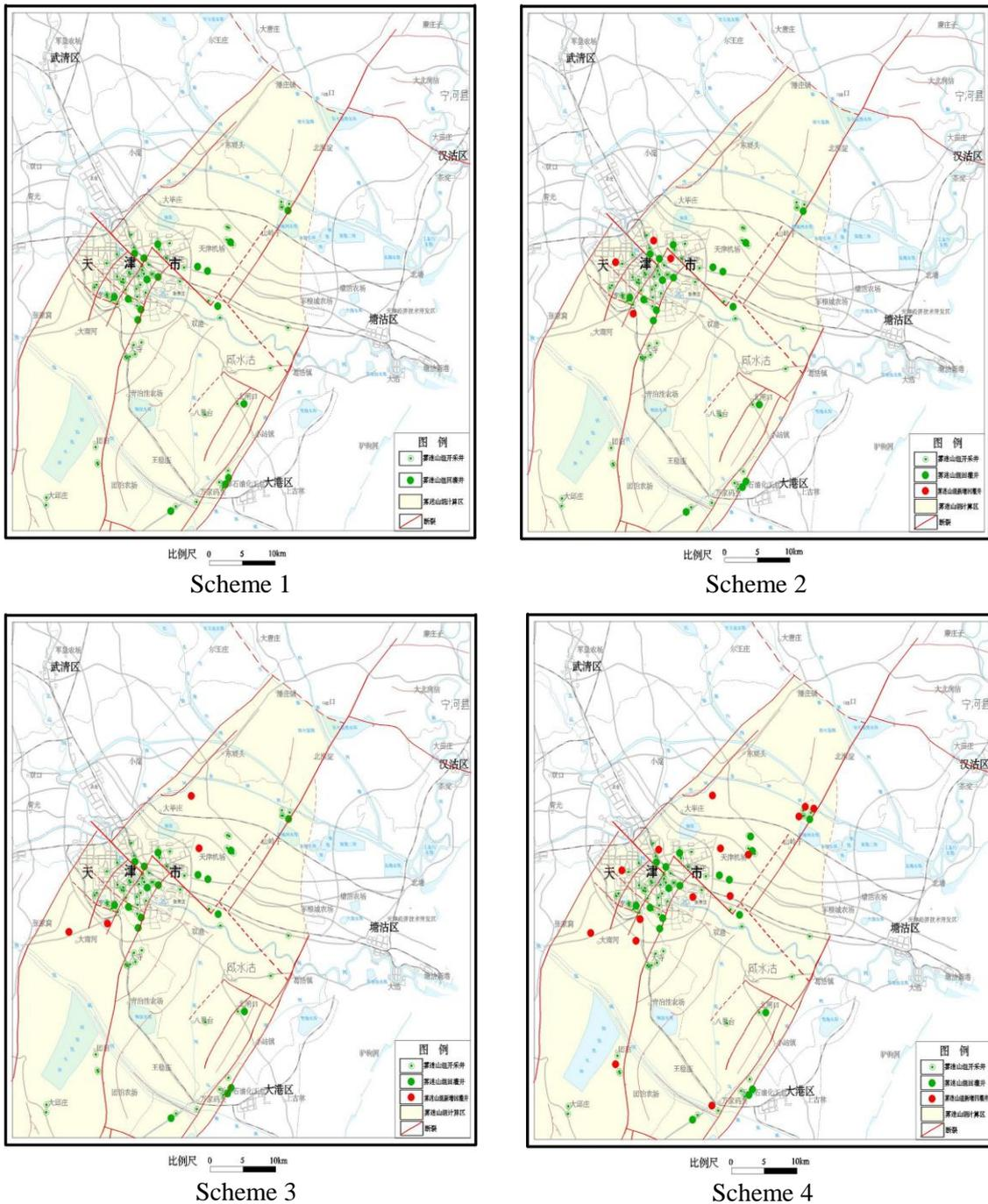
FIGURE 10: Layout of reinjection wells in four different schemes
