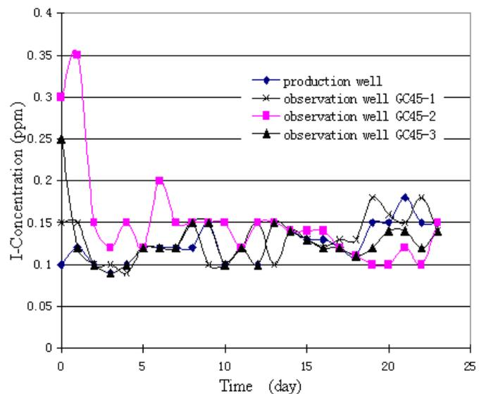
FIGURE 4: The recovery curves of the tracer concentration in the observation wells around WR45.
