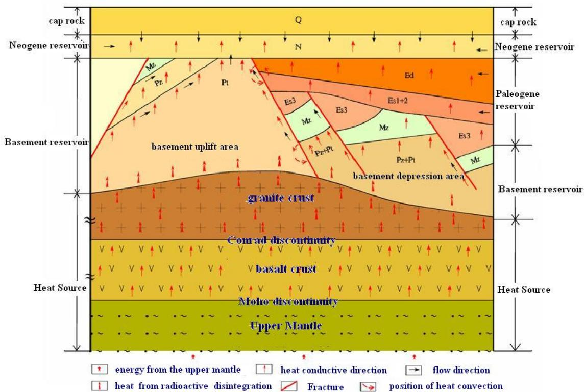
FIGURE 8: Geological geothermal model in Tianjin
