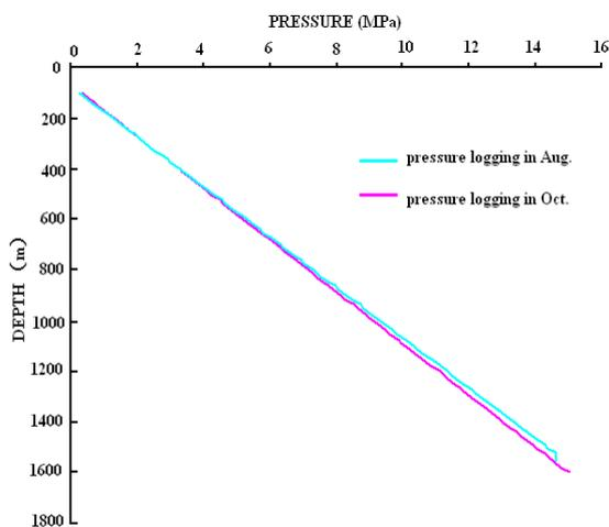
FIGURE 2: Pressure logging curves of reinjection well HX-25
