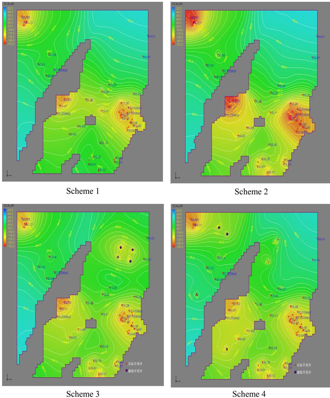
FIGURE 9: Water level contours of Ng group of different schemes in 2034 (Red dots are actual productive wells. Blue dots are virtual new geothermal wells in scheme 3 and 4)
