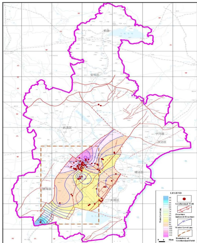
FIGURE 4: Contour of Water levels of Jxw reservoir in Proterozoic, 2007
