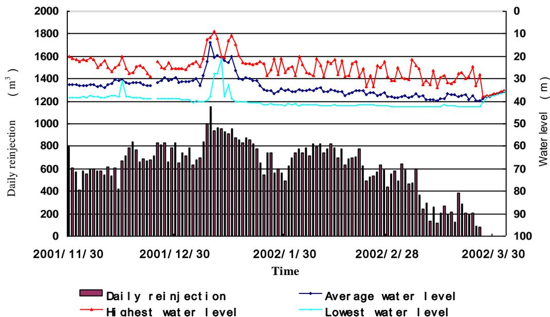
FIGURE 7: reinjection volume and water level changes of a reinjection well in the Xiaotangshan Geothermal Field during the heating season of 2001-2002
