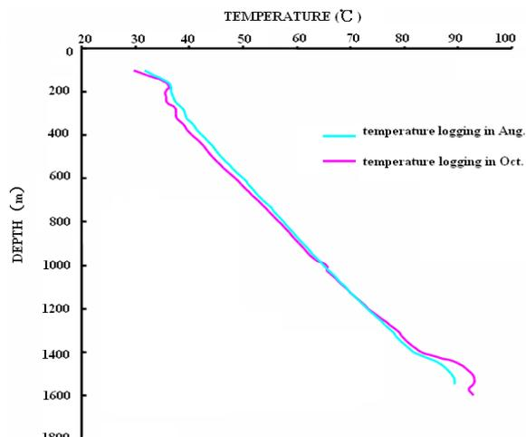
FIGURE 3: Temperature logging curves of reinjection well HX-25
