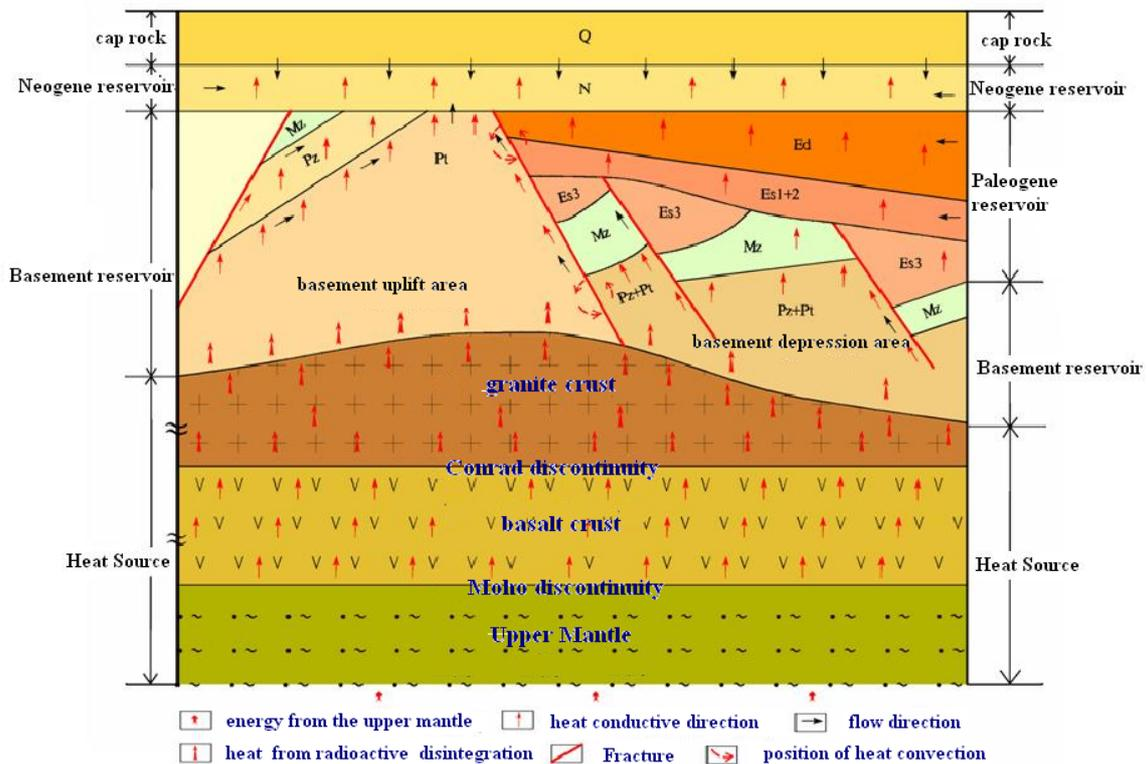
FIGURE 8: Geological geothermal model in Tianjin
