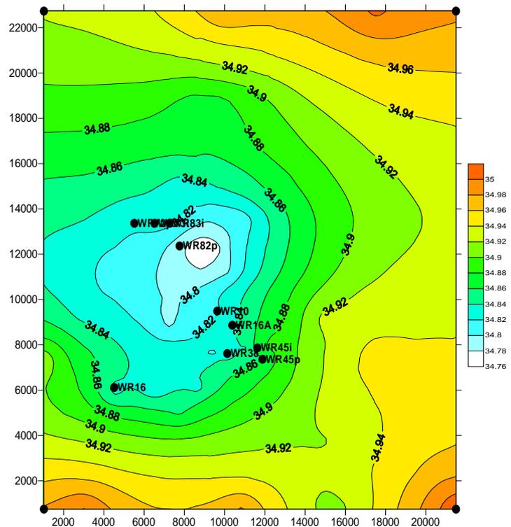
FIGURE 3: Contour map of calculated water level of the dolomite reservoir in Tianjin in Sept. 2013, assuming the reinjection will increase 150%.
