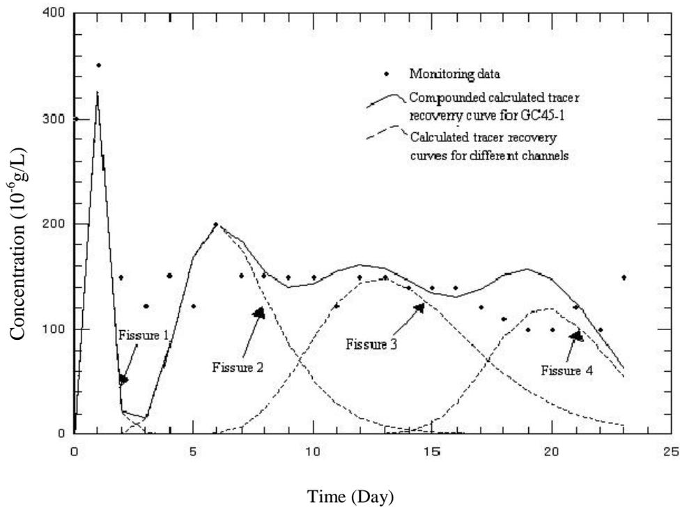
FIGURE 5: Calculated tracer recovery curves for observation well GC45-1. Each dashed line represents a different channel connecting the reinjection and production wells.
