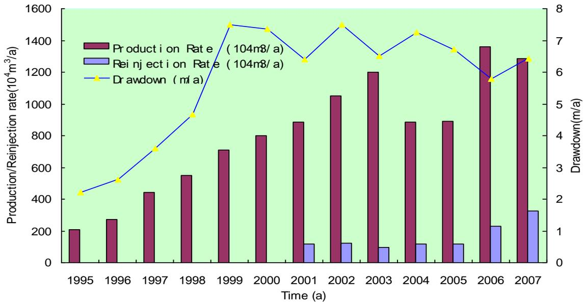
FIGURE 2: The history of water level drawdown v. geothermal water production and reinjection in the dolomite reservoir in the Tianjin urban area in 1995-2007.
