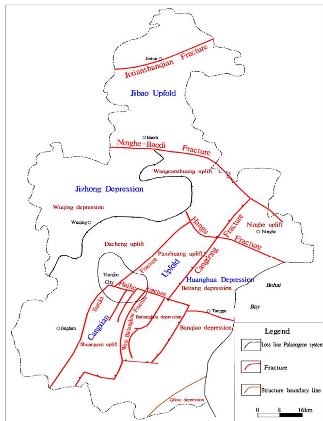
FIGURE 2: Sketch of geological tectonics in Tianjin
