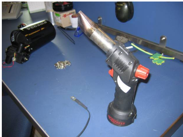
FIGURE 7: Heat gun used to blow hot air to heat shrink sleeves; a cable termination with a heat shrink sleeve can be seen beside the gun
