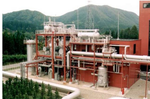
FIGURE 28: Picture of the Selectox H 2 S abatement system at Yanaizu-Nishiyama, Japan (Takahashi and Kuragaki, 2000)
