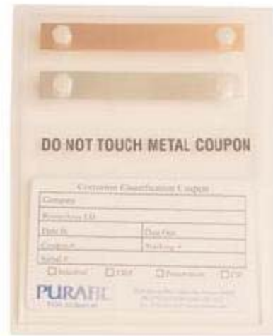
FIGURE 21: Copper and silver coupons for reactivity monitoring (Purafil, n.d.)
