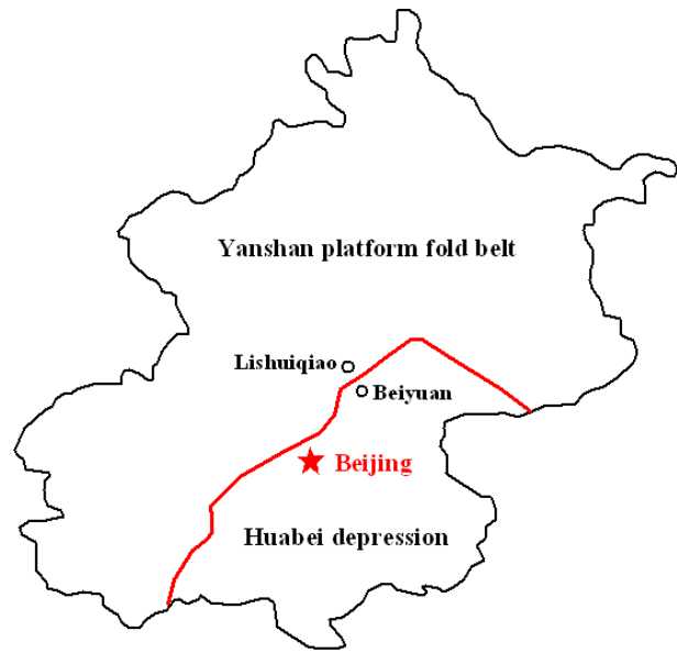
FIGURE 1: The two second-order tectonic units in the Beijing area; also shown is the location of the Lishuiqiao-Beiyuan area
