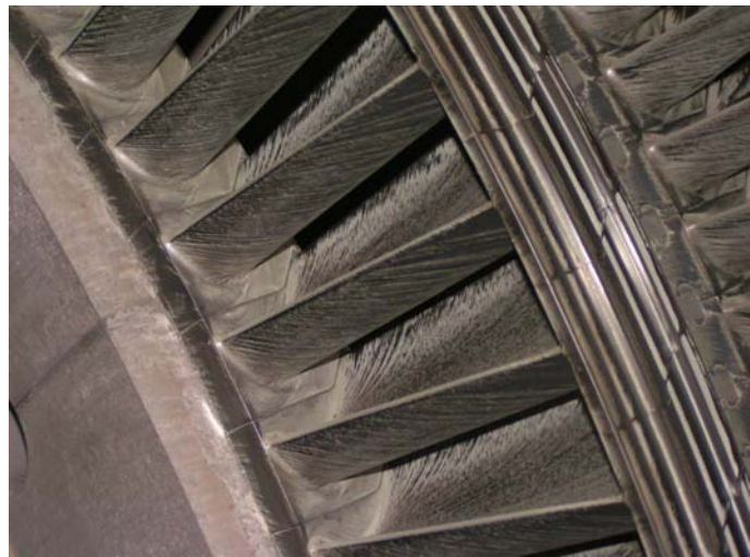
FIGURE 10: Turbine blades erosion
