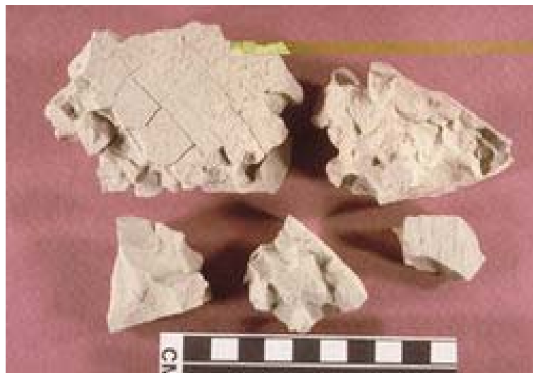
FIGURE 9: Photo showing typical bentonite mud used in drilling mud. Bentonite swells considerably when exposed to water, making it ideal for protecting formations from invasion by drilling fluids.
