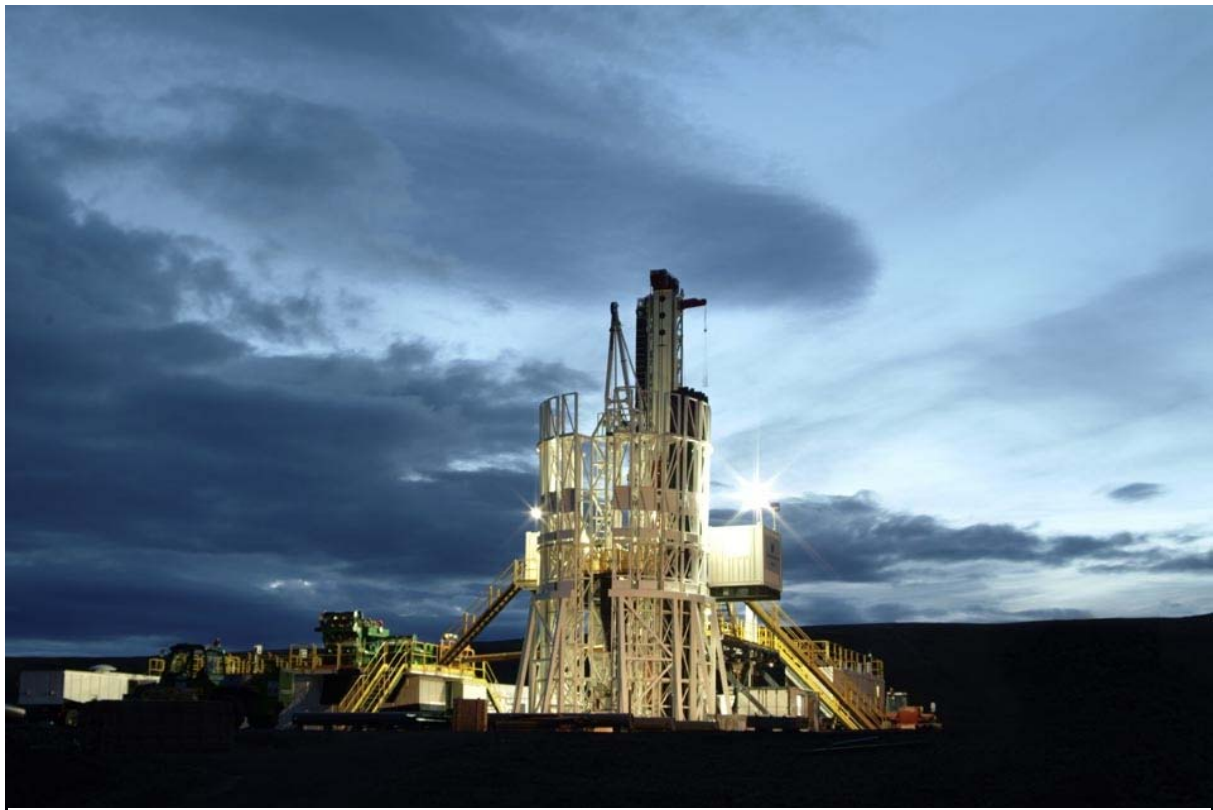
FIGURE 6: Photo of the Icelandic drill rig Geysir, which has a capacity of 200 tonnes
