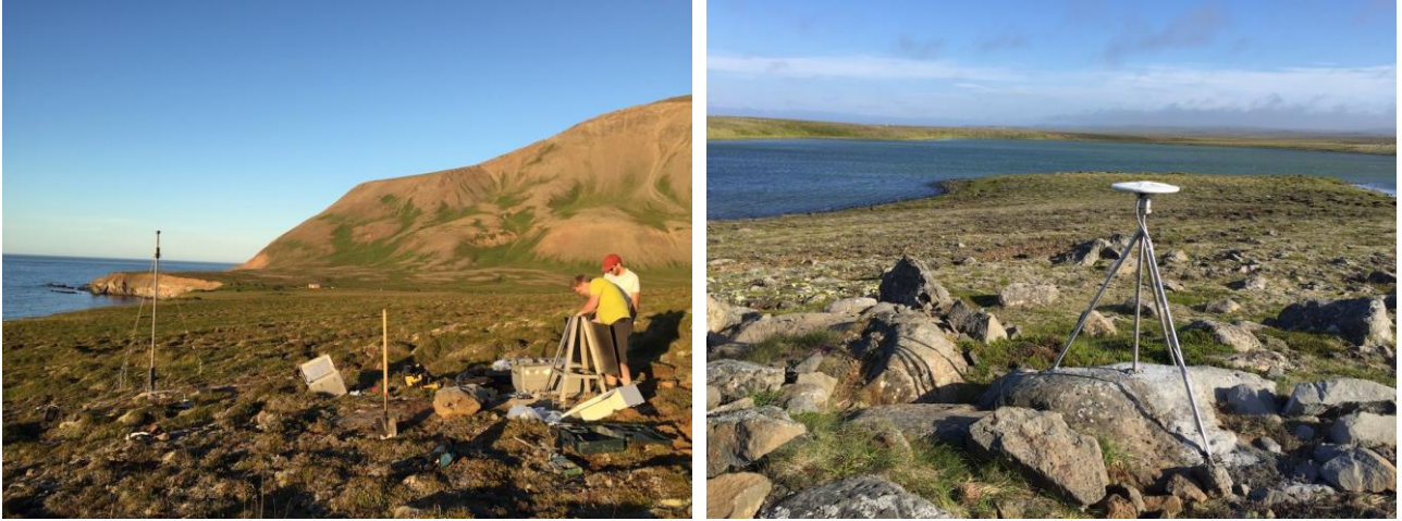
Figure 2. Photos of the CGPS station installation work at GJOC (left) near Gjöfurtá. This isolated station is powered with a solar panel and a wind generator. On the right is the CGPS station HRAC located at the western edge of the network and close to an IMO seismic station.
