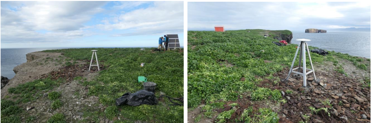
Figure 3. The newest CGPS station in North Iceland is MANA on Lágey, one of the two islands in Mánáreyjar, installed in summer 2018. The photos were taken looking towards North (left) showing the antenna and the solar panel array used to power the station, and towards south (right) with Háey and the north coast in the background.
