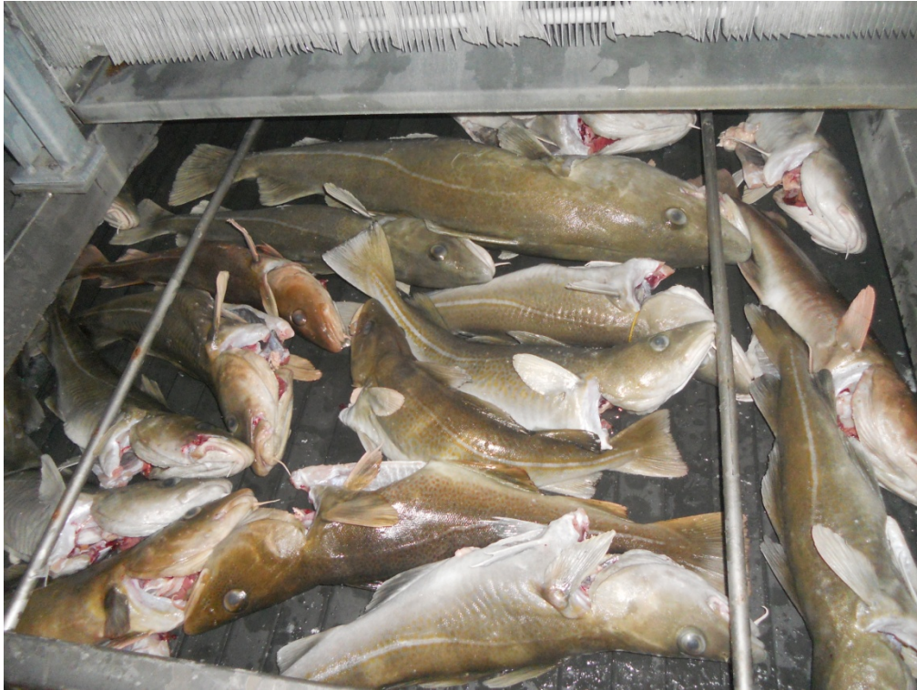
Figure 1. Whole cod fish superchilled by means of combined blast and contact cooling.
