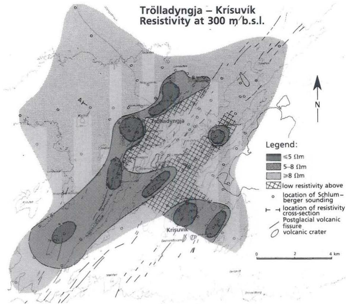
FIGURE 5: Resistivity map of the Krísuvík and Trölladyngja area at 300 m below sea level (Georgsson, 1987)
