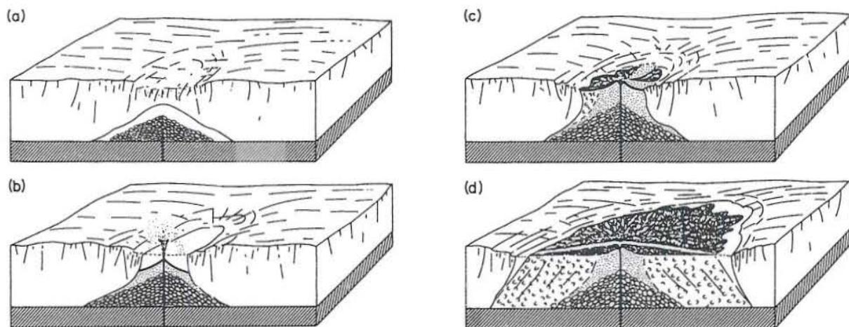
FIGURE 3: Growth of monogenic volcano (by Jones, 1969); a) A pile of pillow lava forms deep in melt water lake; b) Slumping on the flanks of the pillow lava pile produces pillow breccia; c) Hyaloclastite tuffs erupted under shallow water; d) A lava cap progrades across its own delta of foreset breccias
