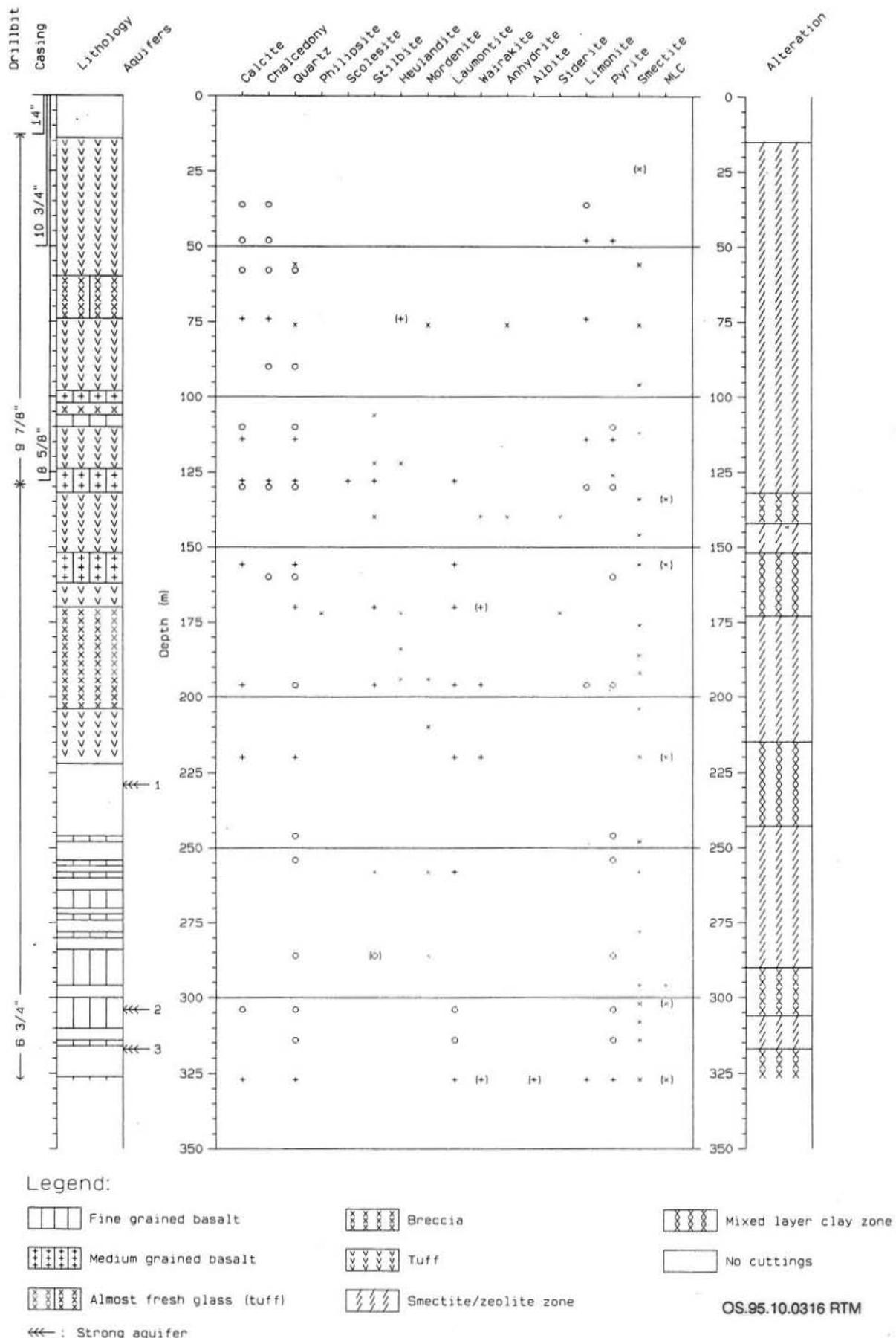
FIGURE 9: Stratigraphy, hydrothermal alteration minerals and alteration zones of well KR-9
