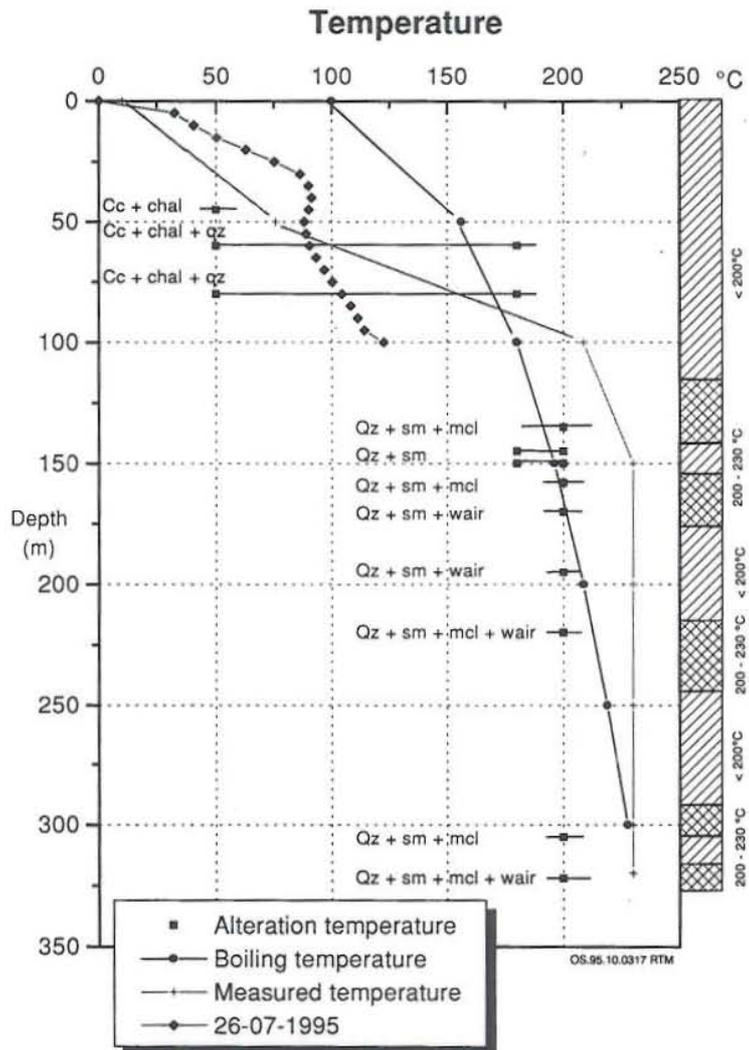
FIGURE 11: Correlation of measured temperature and alteration temperature in well KR-9
