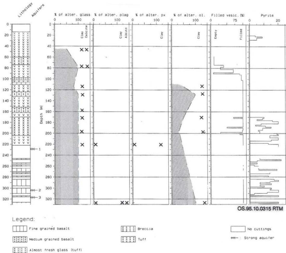
FIGURE 8: Lithology of well KR-9 in Krísuvík, alteration state of primary minerals, glass, filling of vesicles and relative abundance of pyrite (0 = absent; 1-10 = common; 11-20 = abundant; >20 = very abundant)
