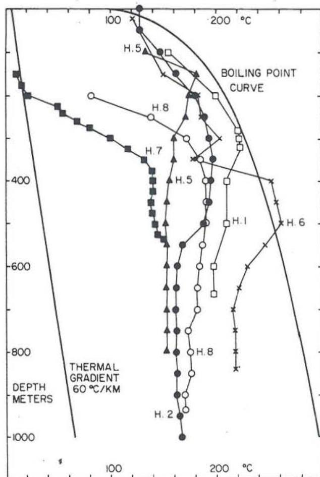
FIGURE 6: Temperature logs of deep wells in the Krísuvík area (Arnórsson et al. 1975)
