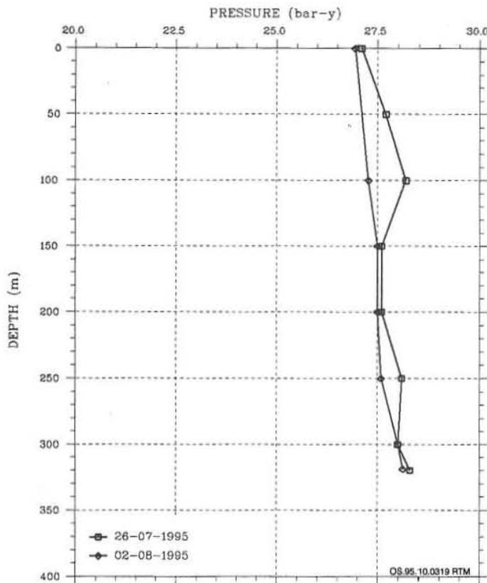
FIGURE 13: Pressure logs of well KR-9
