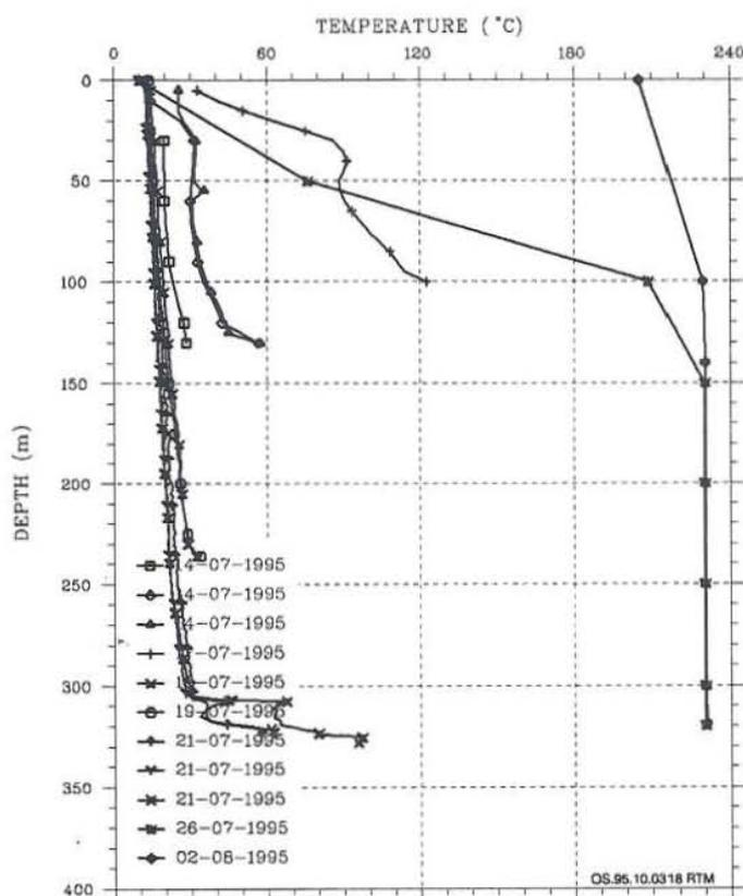
FIGURE 12: Temperature logs of well KR-9
