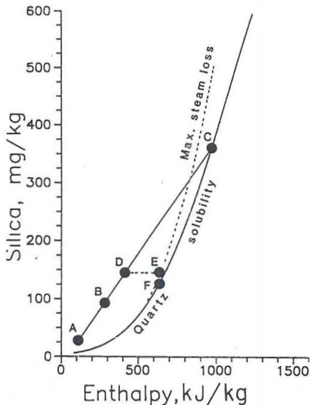
FIGURE 7: Silica-enthalpy diagram illustrating use in calculating silica mixing model temperatures (Fournier, 1977)
