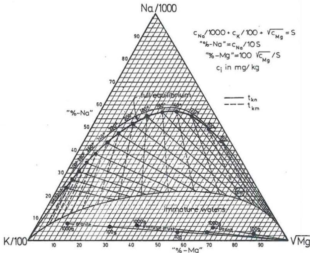
FIGURE 8: Blank diagram for the evaluation of Na-K and K-Mg equilibrium temperatures (Giggenbach, 1988)
