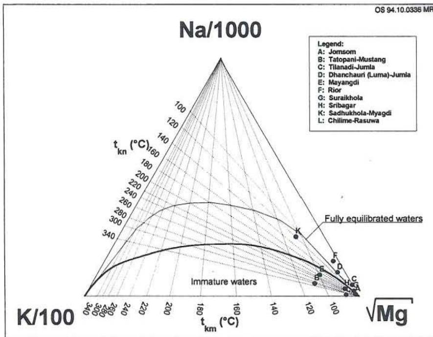
FIGURE 11: Diagram for the evaluation of Na-K and K-Mg equilibrium temperature of the thermal springs
