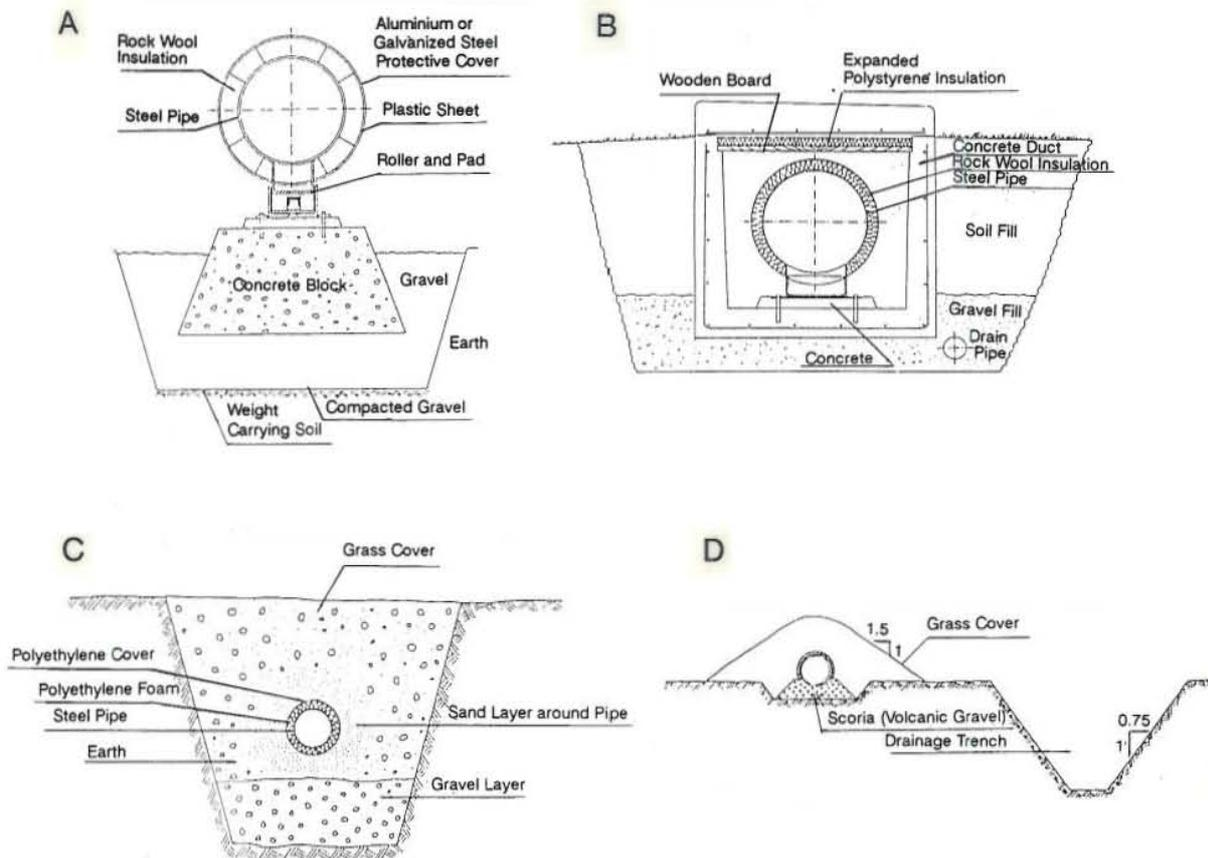
FIGURE 1.13: Examples of above and below ground pipelines, a) Above ground pipeline with sheet metal cover; b) Steel pipe in concrete tunnel; c) Steel pipe with polyurethane insulation and polyethylene cover; d) Asbestos cement pipe with earth and grass cover
