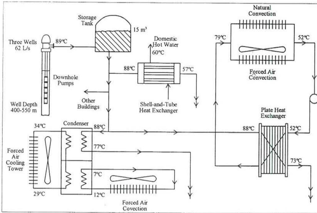
FIGURE 1.4: Oregon Institute of Technology heating and cooling system
