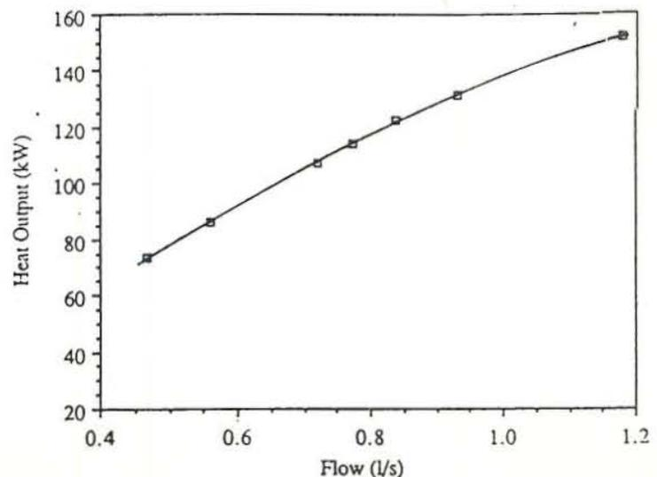
FIGURE 2.13: Heat output vs. flow rate
