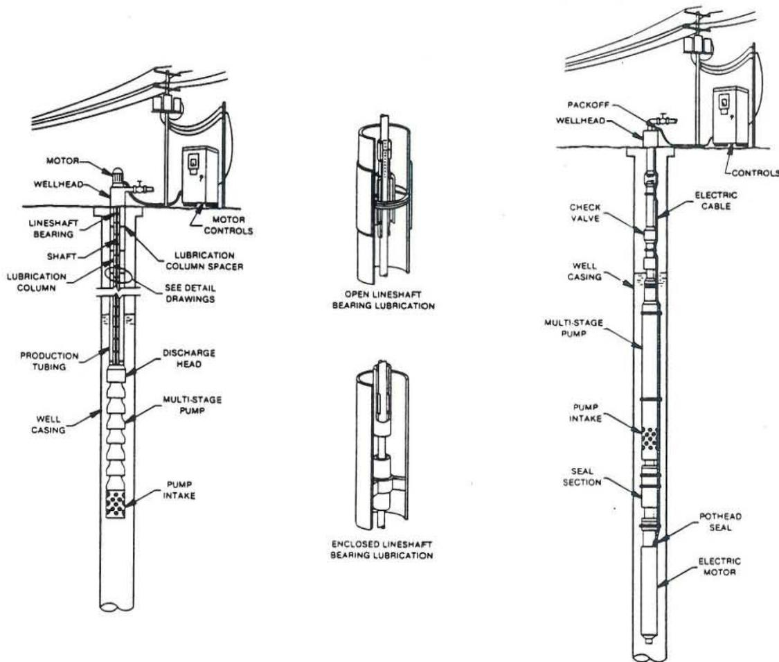
FIGURE 1.10: Line shaft pump
