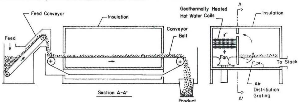
FIGURE 1.8: Continuous belt dehydration plant, schematic
