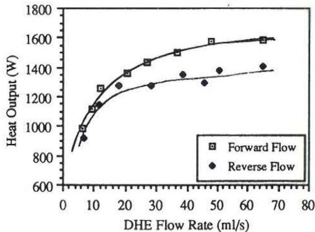
FIGURE 2.16: Heat output vs. DHE flow (32 mm promoter) (Cross flow rate 25.8 ml/s)
