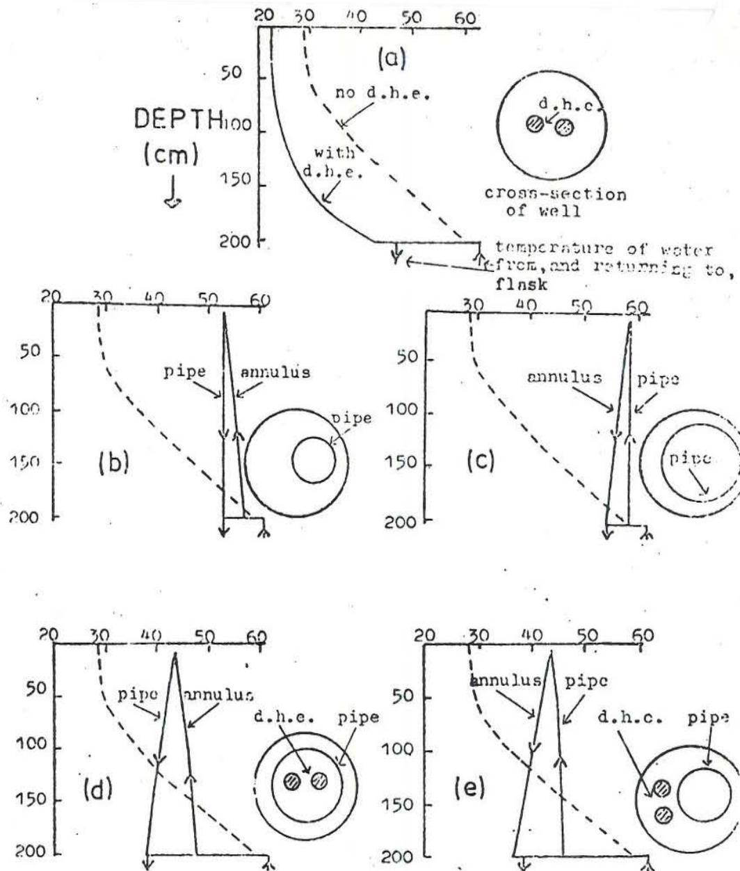
FIGURE 2.9: Characteristic temperature and flow regimes observed in a laboratory model of a well; configuration of convection promoting pipe and/or DHE is shown in the cross-section in each case
