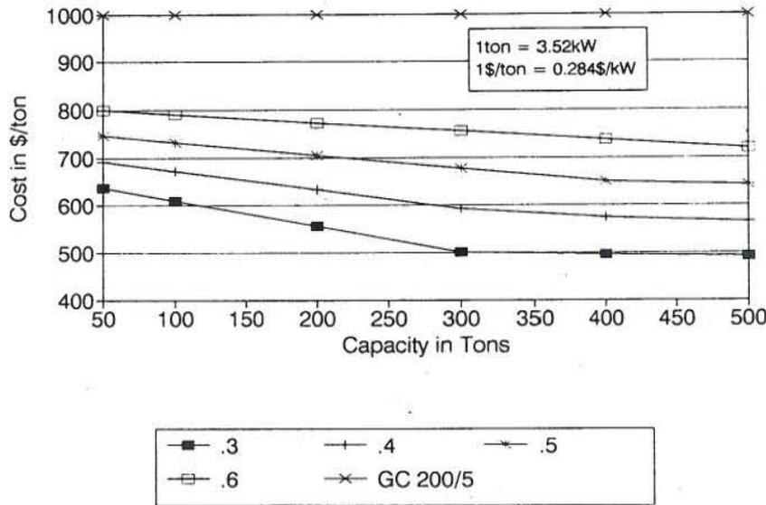
FIGURE 5.20: Hybrid system cost - 60°F (15.5°C) soil
