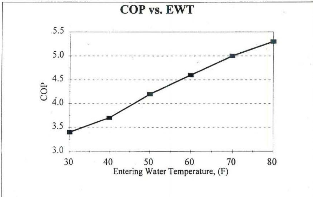
FIGURE 5.13: COP for a 3 ton (10.5 kW) GSHP
