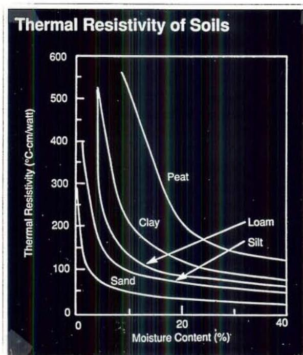
FIGURE 5.26: Ground loops function more efficiently in wetter soils where thermal resistivity is lower
