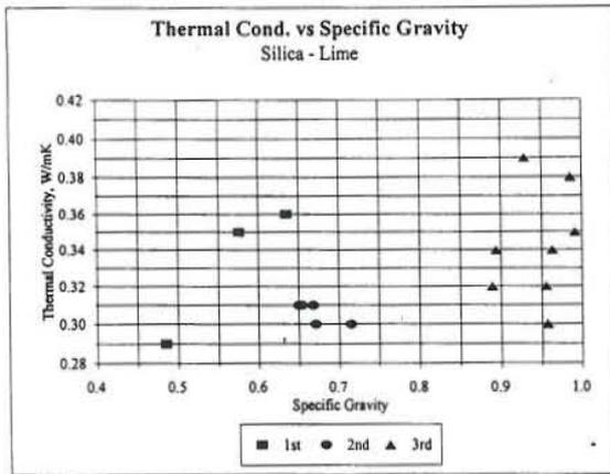
Figure 7. Specific gravity vs. thermal conductivity of selected silica-lime samples.
