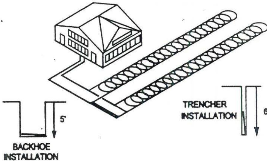
FIGURE 5.2: Slinky coil ground-coupled heat pump system
