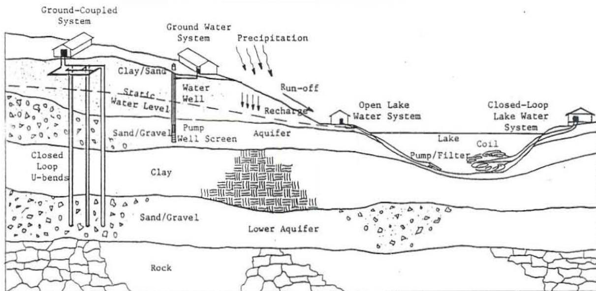
FIGURE 5.9: Ground-coupled, groundwater and two lake-water heat pump systems in a typical hydrogeological formation
