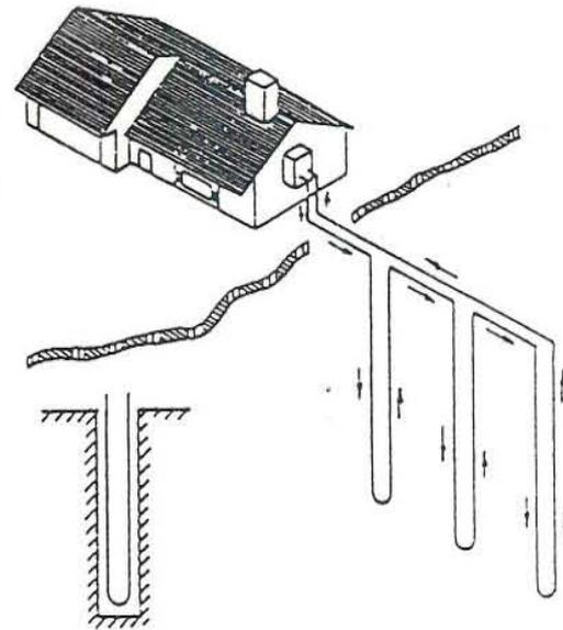
FIGURE 1.16: Typical ground-source heat pump installations
