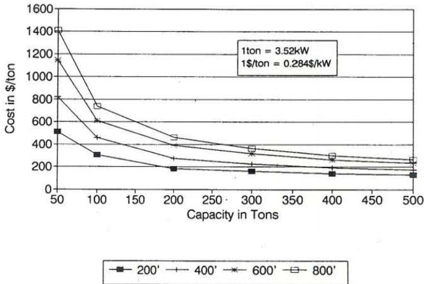
FIGURE 5.19: Groundwater system cost (1 well - 60°F (15.5°C) water)
