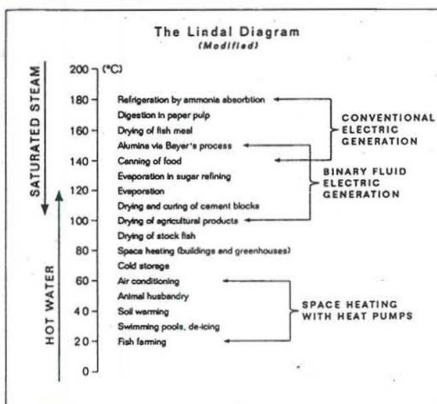
FIGURE 6.1: The Lindal diagram on typical fluid temperatures for direct applications of geothermal resources (modified from Lindal, 1973)
