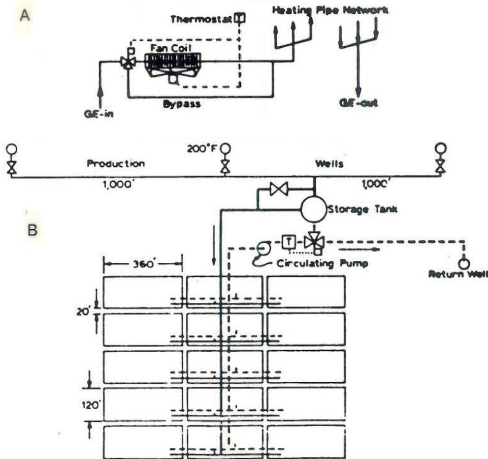
FIGURE 3.4: a) Unit heating system design (three per house); b) Six-hectar greenhouse complex
