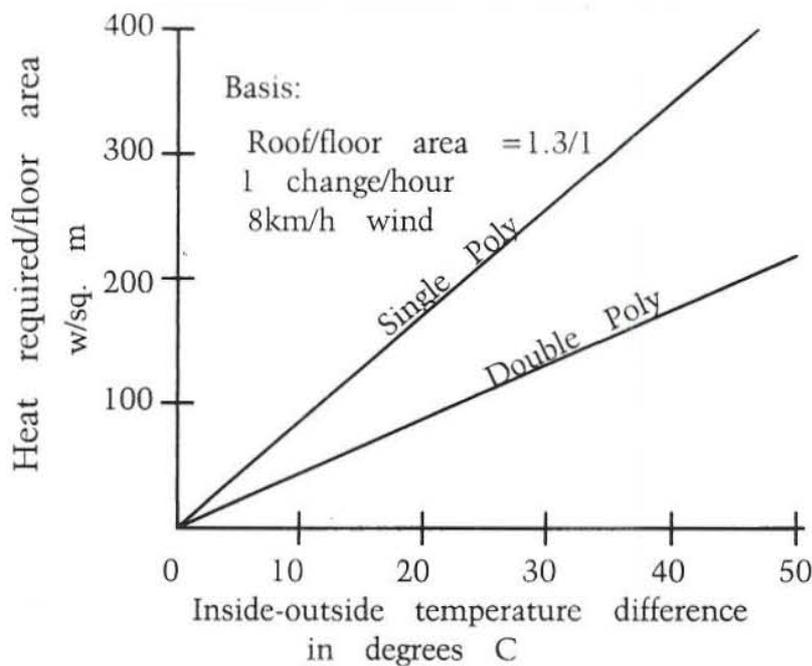
FIGURE 3.2: Example of heat requirement for greenhouses in La Grande, Oregon (outside design temperature = 1°F [-17°C])
