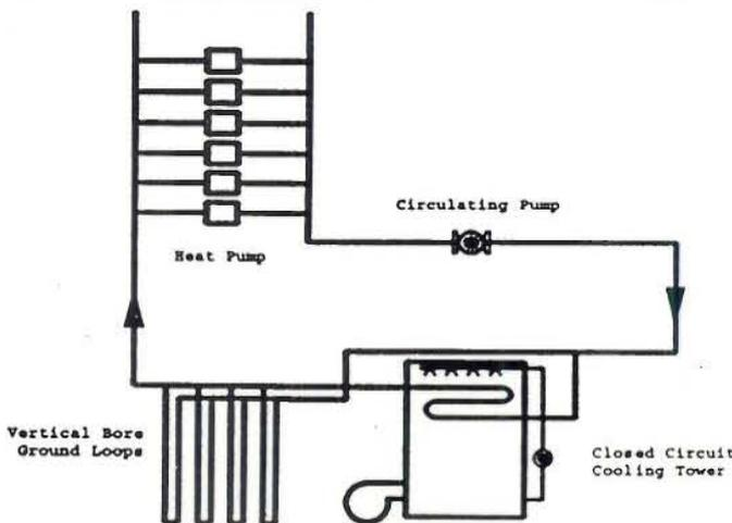
FIGURE 5.18: Hybrid ground-coupled heat pump system
