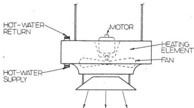
FIGURE 3.9: Vertical hot water unit heater
