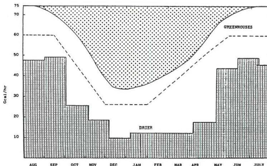
FIGURE 3.3: Geothermal energy consumed by greenhouses and drier at Mt. Amiata, Italy
