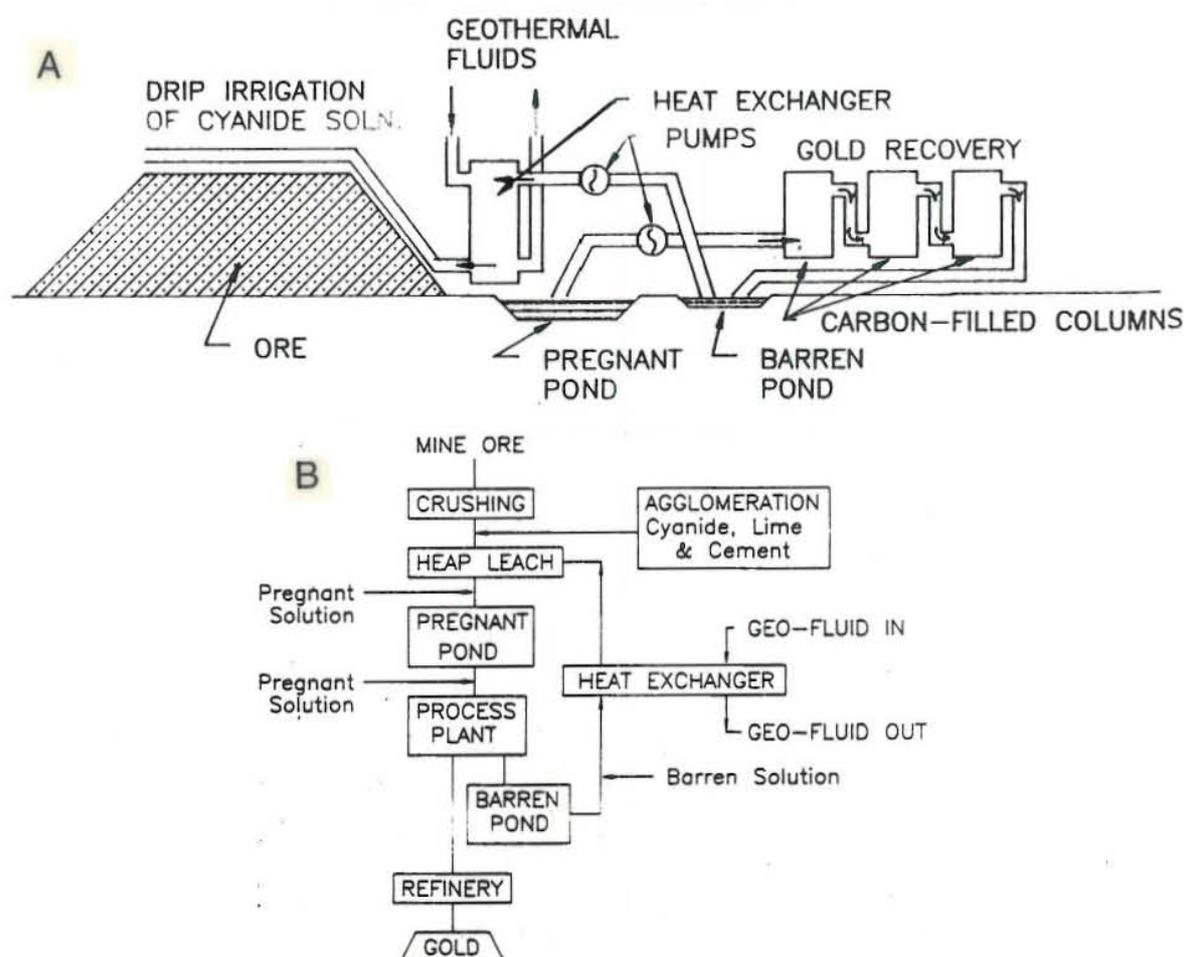
FIGURE 6.3: a) Idealized thermally enhanced heap leach (Trexler et al., 1990);
