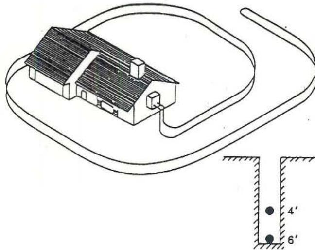
FIGURE 5.5: Series vertical ground heat exchanger (source: Oklahoma State University):
