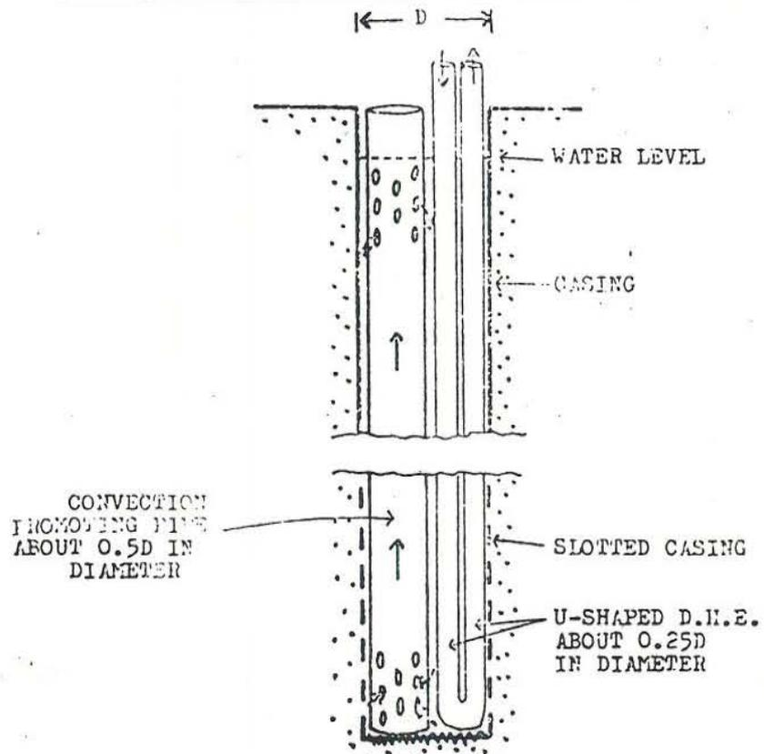
FIGURE 2.7: Scheme for optimizing the heat output of a DHE
