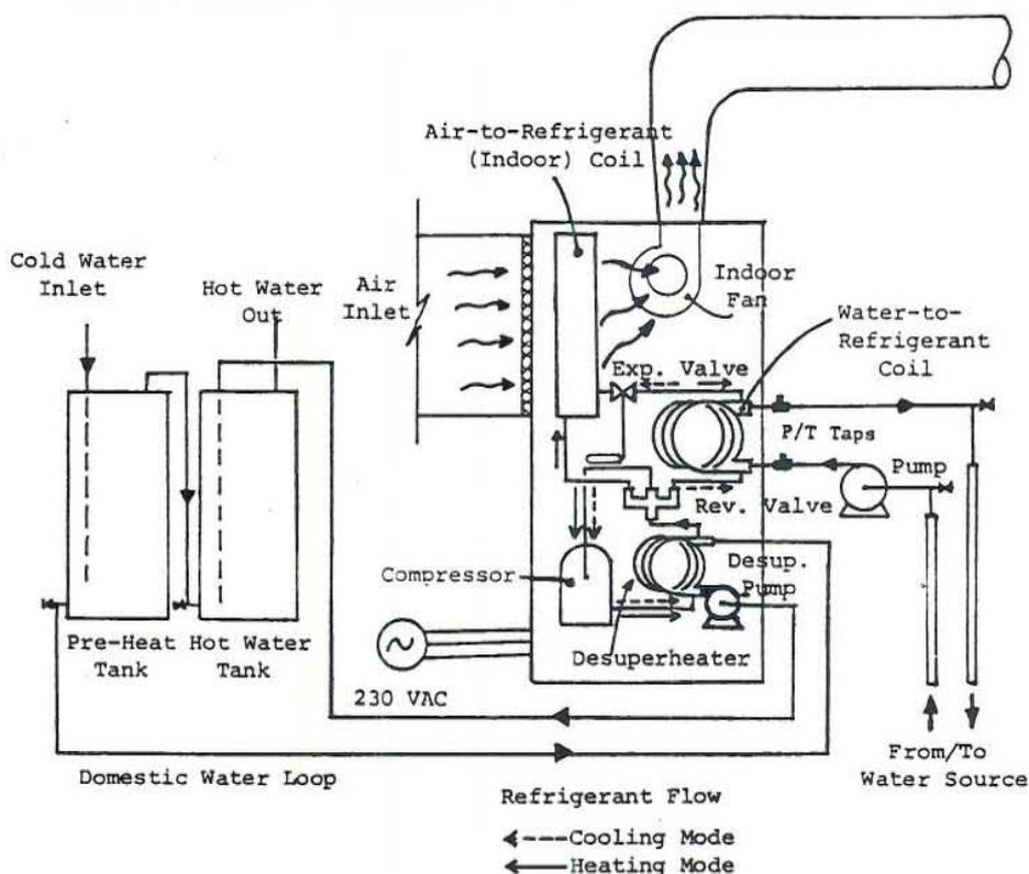
FIGURE 5.14: Typical water-to-air heat pump arrangement
