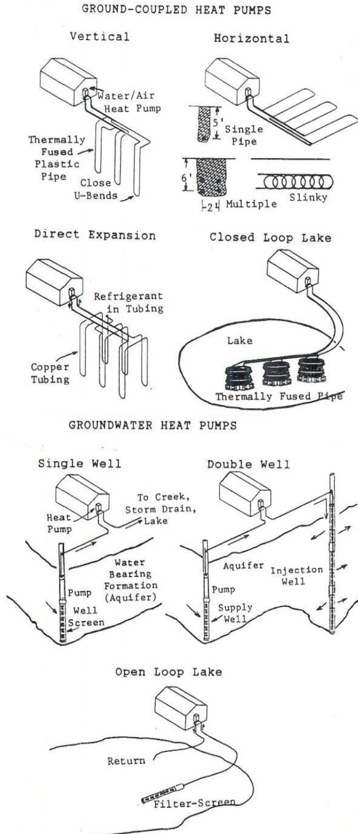
FIGURE 5.1: Ground-source heat pump types
