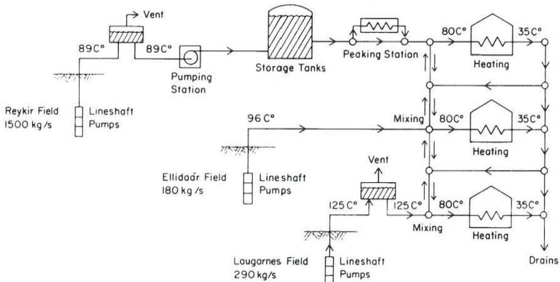
FIGURE 1.5: Reykjavik district heating system (prior to the Nesjavellir connection)
