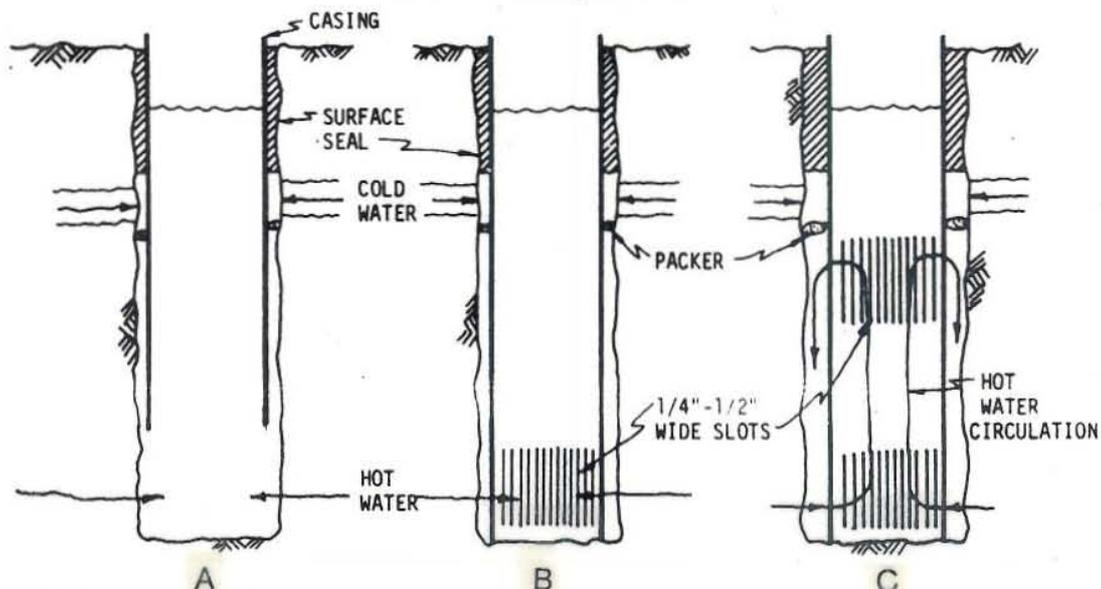
FIGURE 2.4: Well completion systems for downhole heat exchangers (type c preferred)
