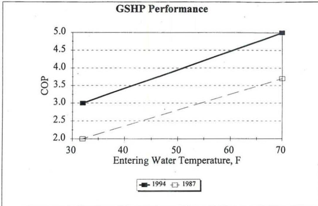
FIGURE 5.10: GSHP performance improvements from 1987 to 1994 for heating mode
