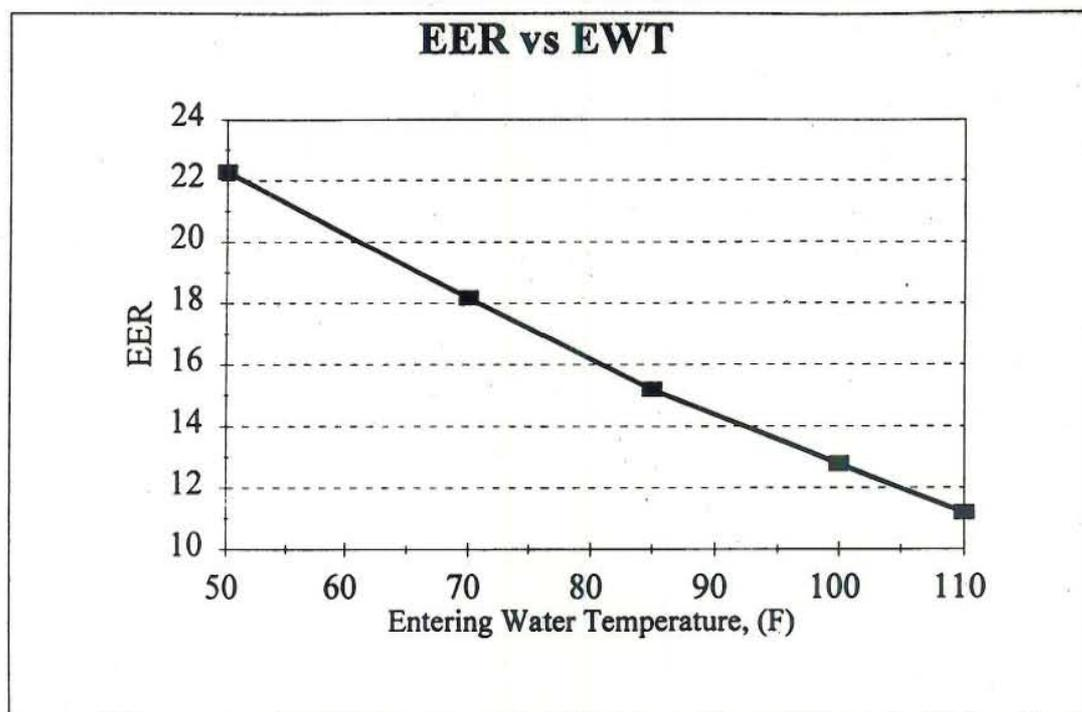
FIGURE 5.12: EER for a 3 ton (10.5 kW) GSHP
