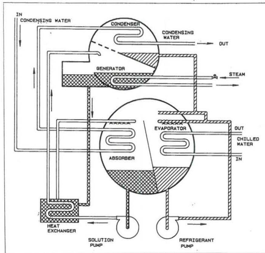
FIGURE 6.5: Lithium-bromide absorption refrigeration
