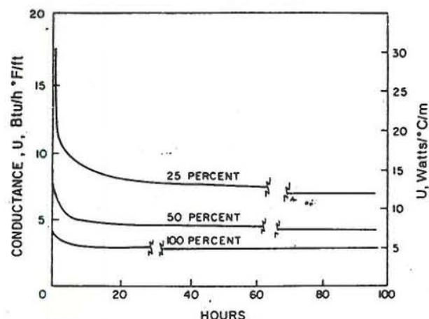
Figure 5.24: Typical runs of heat injection to earth with three duty cycle
