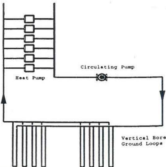
FIGURE 5.17: Ground-coupled heat pump system
