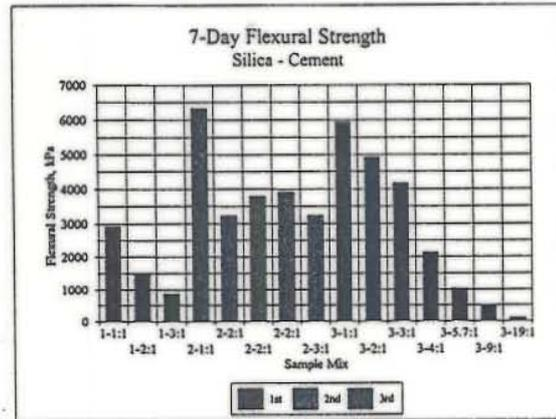
Figure 6. Flexural strength of selected silica-cement mixtures.
