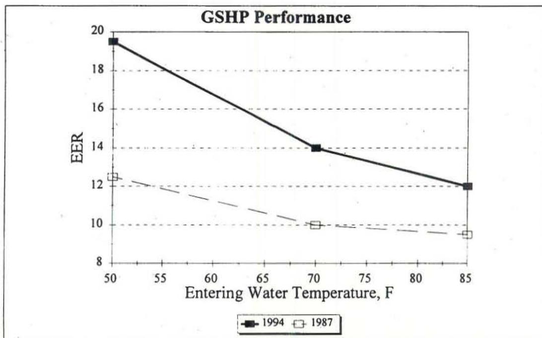
FIGURE 5.11: GSHP performance improvements from 1987 to 1994 for cooling mode
