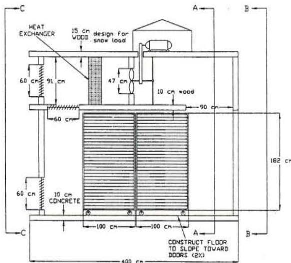
Figure 2a. Detailed drawing of tunnel dehydrator.
