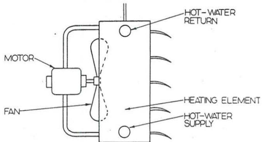
FIGURE 3.8: Horizontal hot water unit heater
