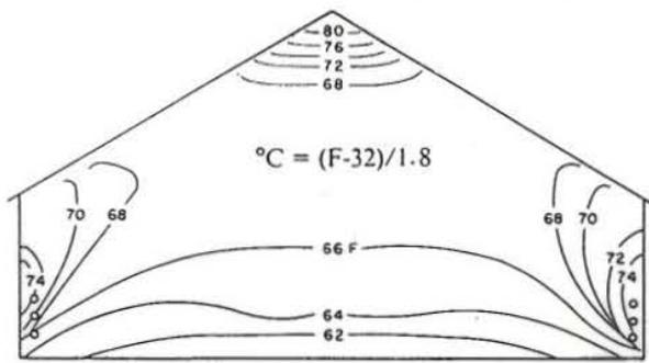
FIGURE 3.7: Temperature profiles in a greenhouse heated with radiation piping along the side walls
