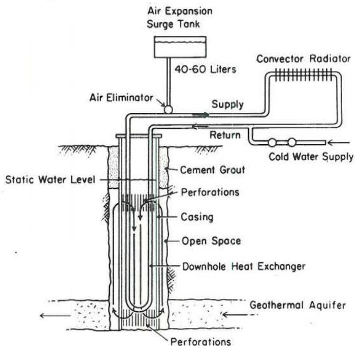
FIGURE 1.15: Downhole heat exchanger (typical of Klamath Falls, Oregon)
