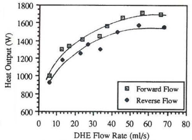
FIGURE 2.17: Heat output vs. DHE flow (32 mm promoter) (Cross flow rate 31.4 ml/s)
