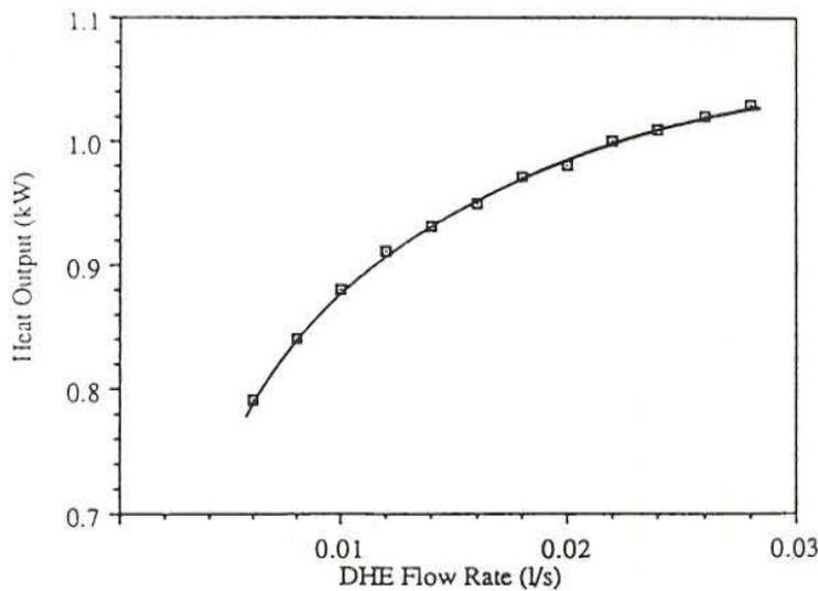
FIGURE 2.14: Typical output curve for a DHE (taken from numerical data by Pan, 1983)
