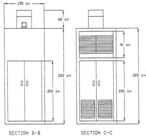
Figure 2b. Cross sections of dehydrator.
