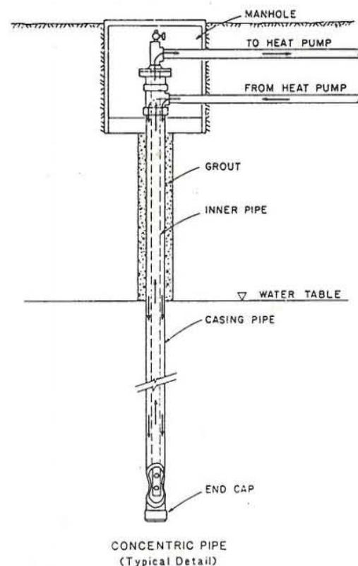
FIGURE 5.22: Concentric pipe configuration for vertical heat exchanger
