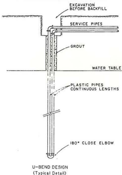
FIGURE 5.23: Two pipe side-by-side configuration for vertical heat exchanger
