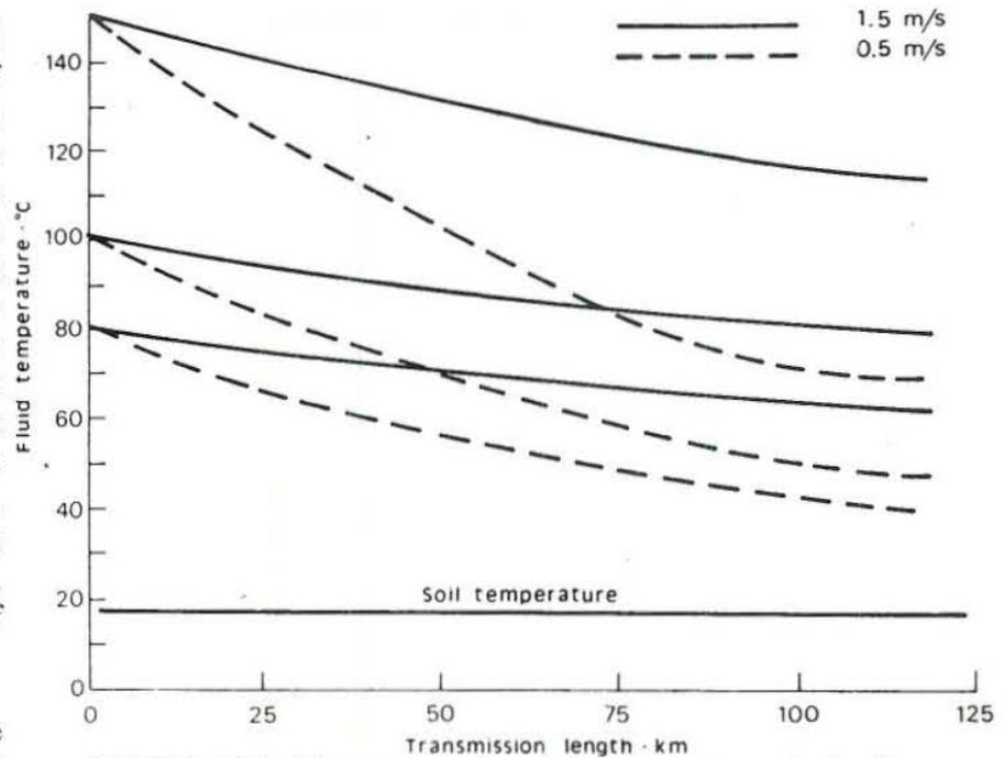
FIGURE 1.12: Temperature drop in hot water transmission line
