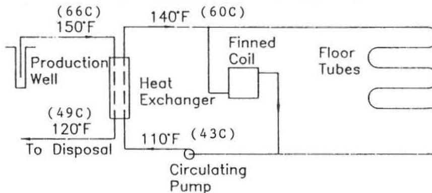
FIGURE 3.6: Heat exchanger schematic
