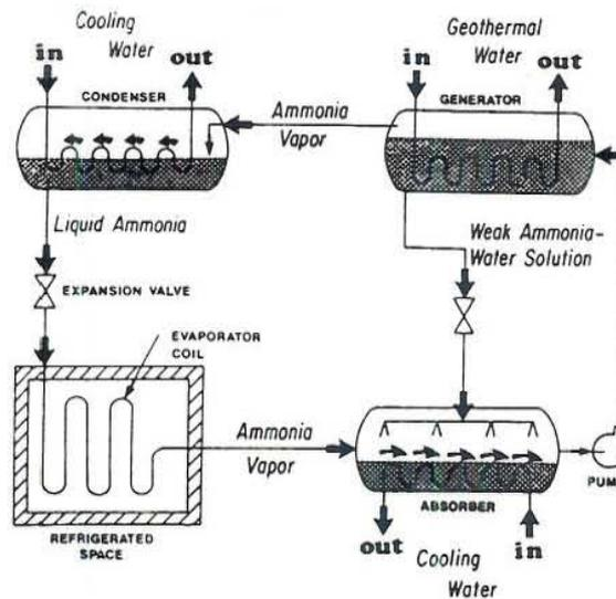
FIGURE 1.17: Geothermal absorption refrigeration cycle
