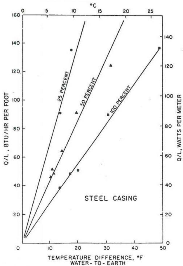
FIGURE 5.25: Earth absorption rate,  $Q/L$  plotted vs. average water to earth temperature difference for 25, 50 and 100% run time (duty cycle)
