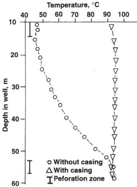
FIGURE 2.5: Temperature vs. depth for a geothermal well (with and without perforations)
