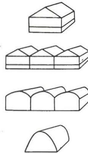
FIGURE 3.5: Structural shapes of commercial greenhouses
