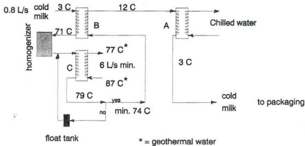
FIGURE 6.7: Medo-Bel milk pasteurization process
