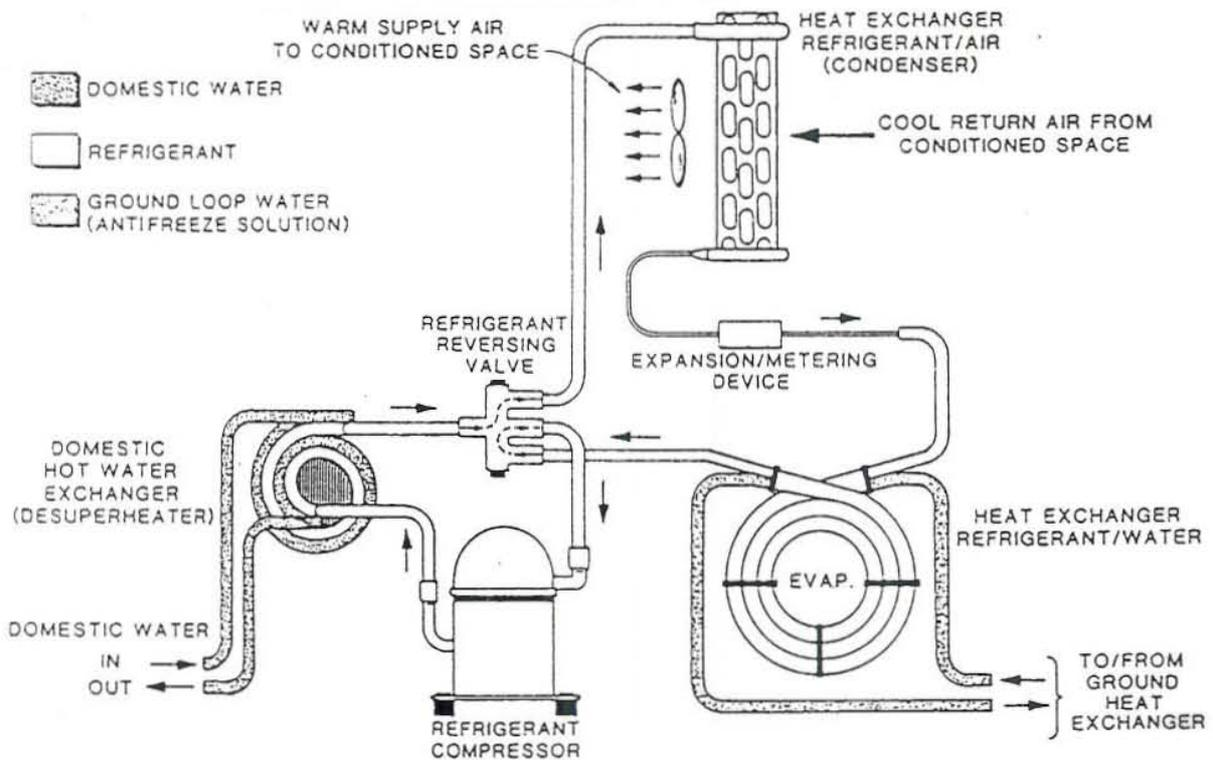
FIGURE 5.8: Heating cycle (source: Oklahoma State University)
