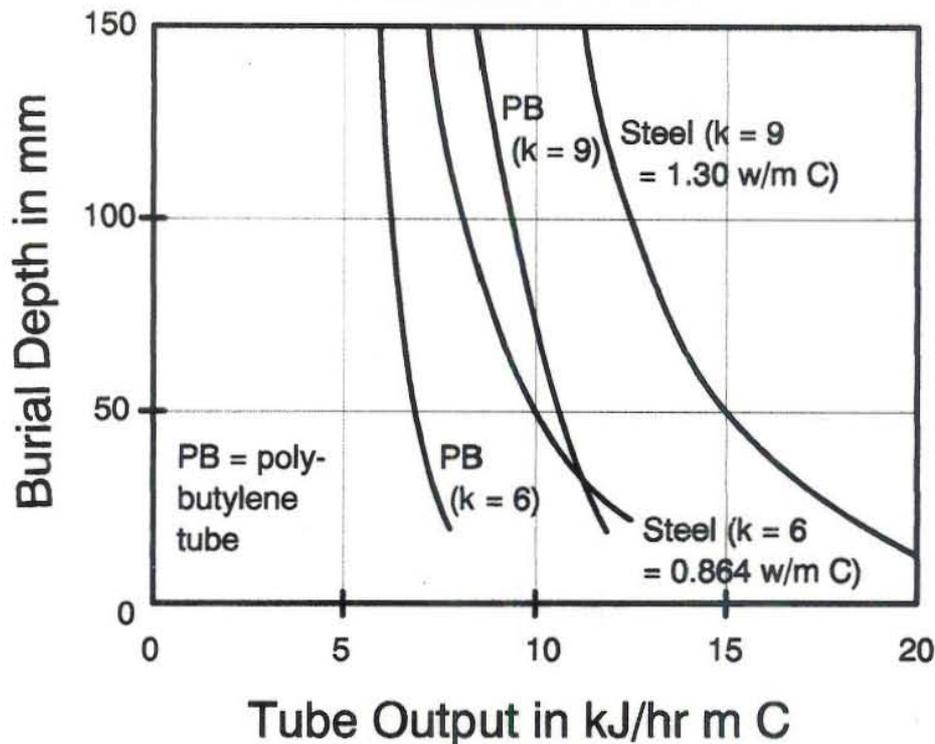
FIGURE 3.12: Heat output for radiant floor system
