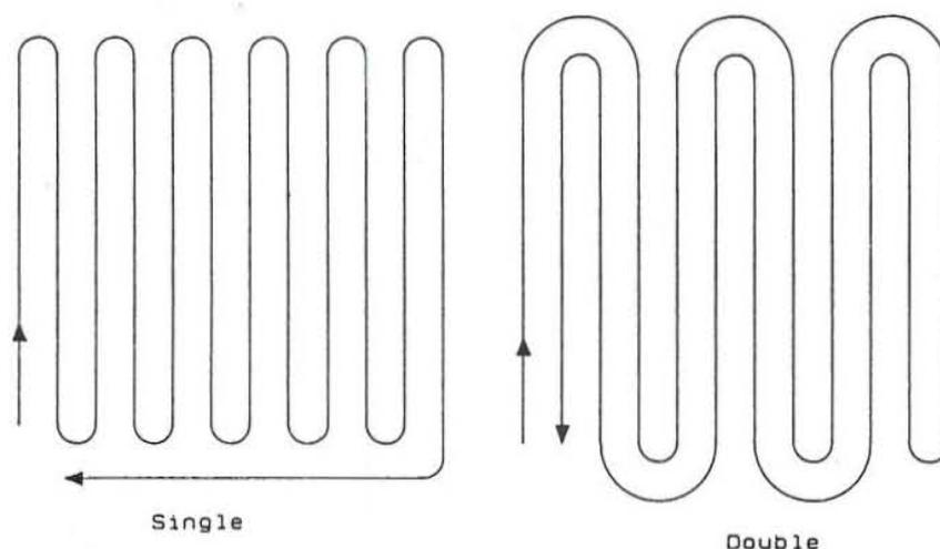
FIGURE 3.11: Single and double serpentine piping layout
