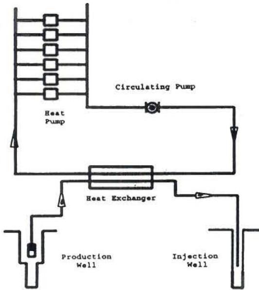
FIGURE 5.16: Groundwater heat pump system
