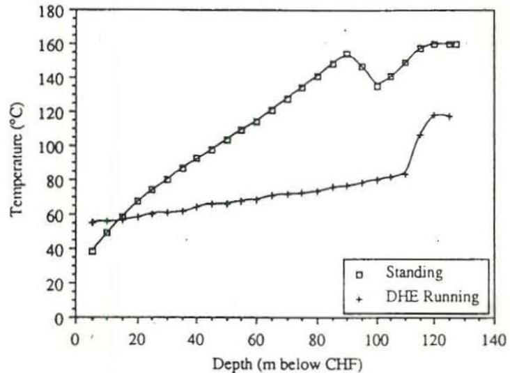
FIGURE 2.11: Downhole temperature
