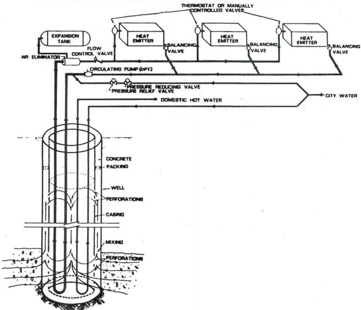
FIGURE 2.1: Typical downhole heat exchanger system (Klamath Falls, OR)
