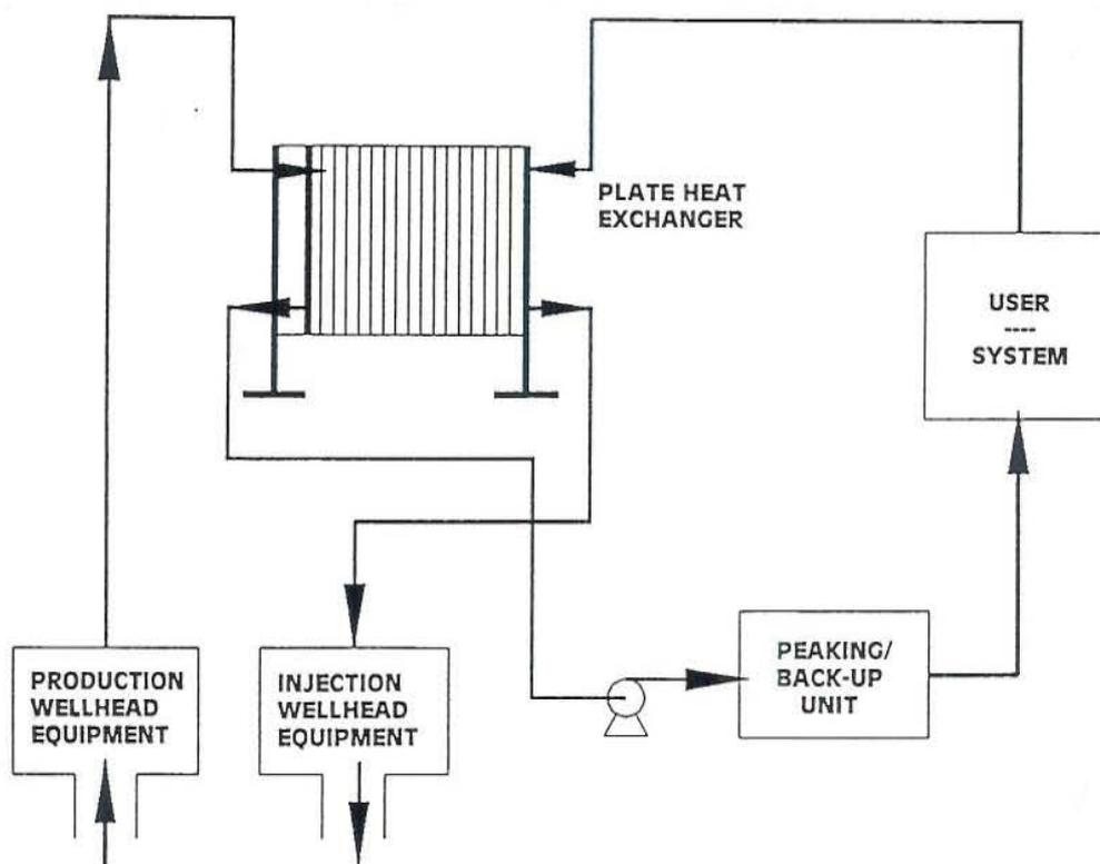
FIGURE 1.9: Geothermal direct utilization system using a heat exchanger
