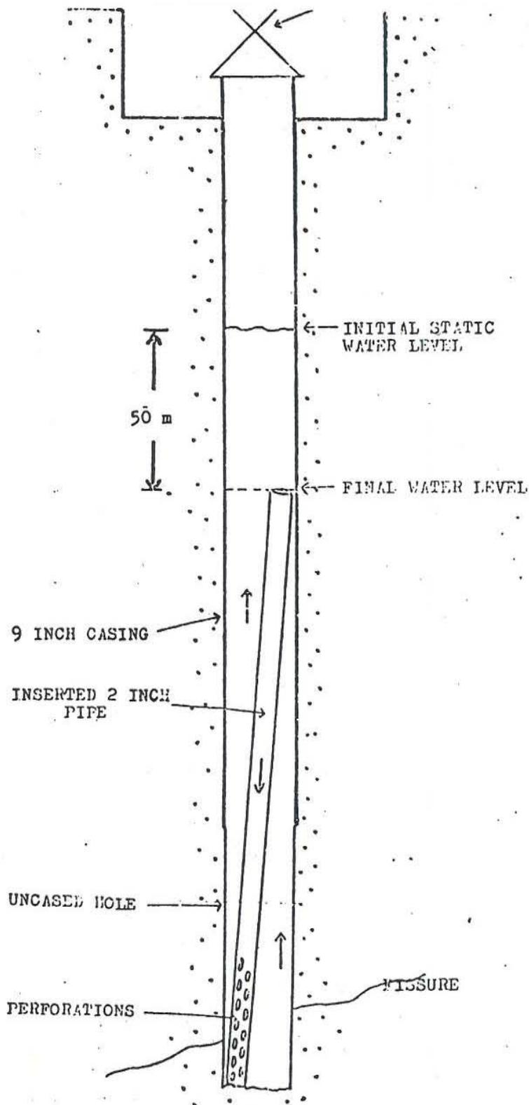
FIGURE 2.10: Scheme for promoting convection in a geothermal power well
