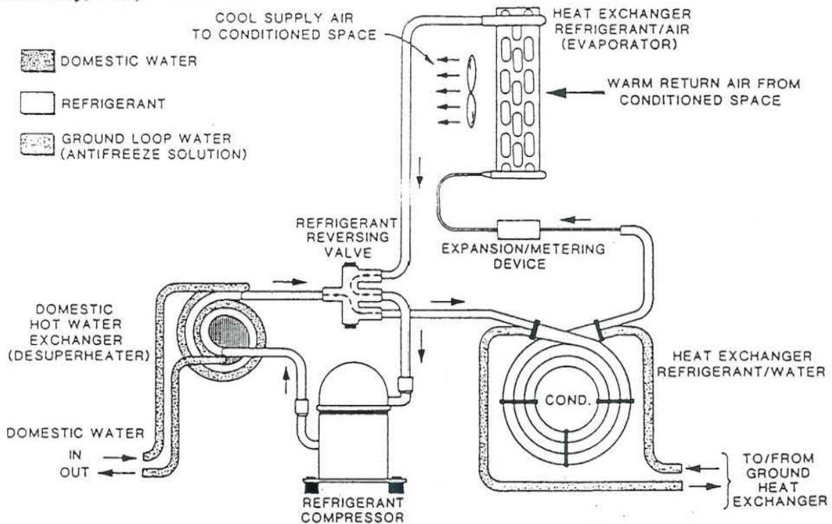
FIGURE 5.7: Cooling cycle (source: Oklahoma State University)
