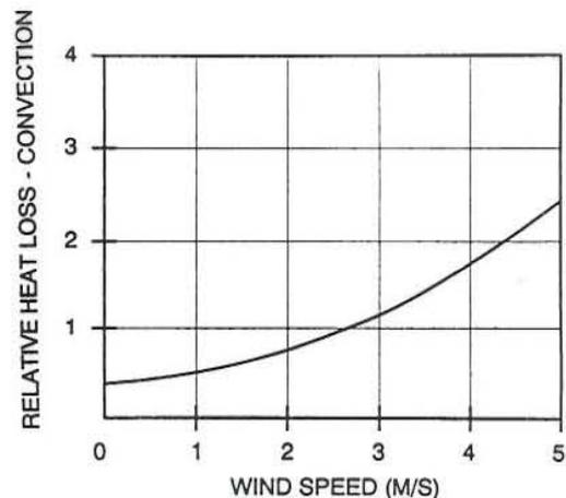
FIGURE 4.4: Plot of relative convective heat loss vs. wind speed
