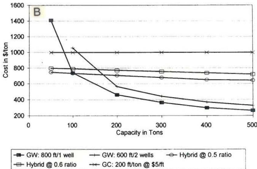
FIGURE 5.21: Ground-source system costs, 60°F water or soil, a) Low case; b) High case
