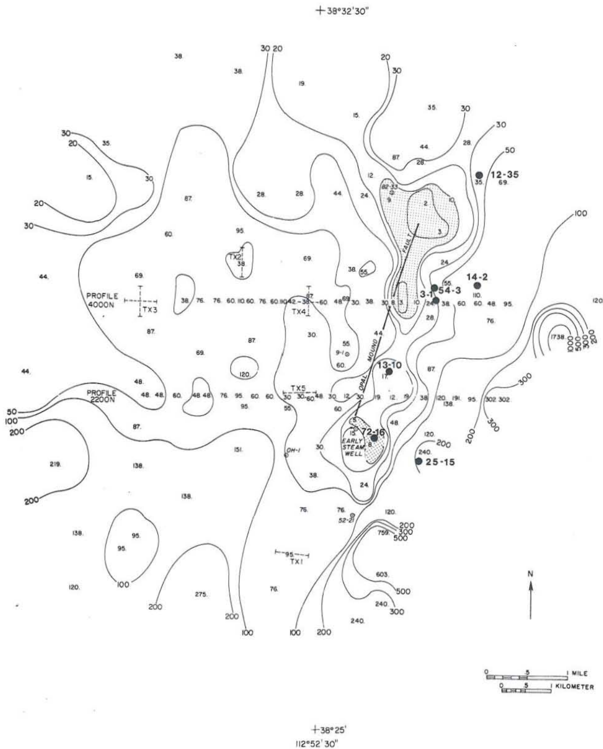
Figure 10. CSAMT apparent resistivity map of Roosevelt Hot Springs KGRA. Frequency = 977 Hz. Areas less than 10 \Omega -m are shaded. (After Sandberg and Hohmann, 1980).
