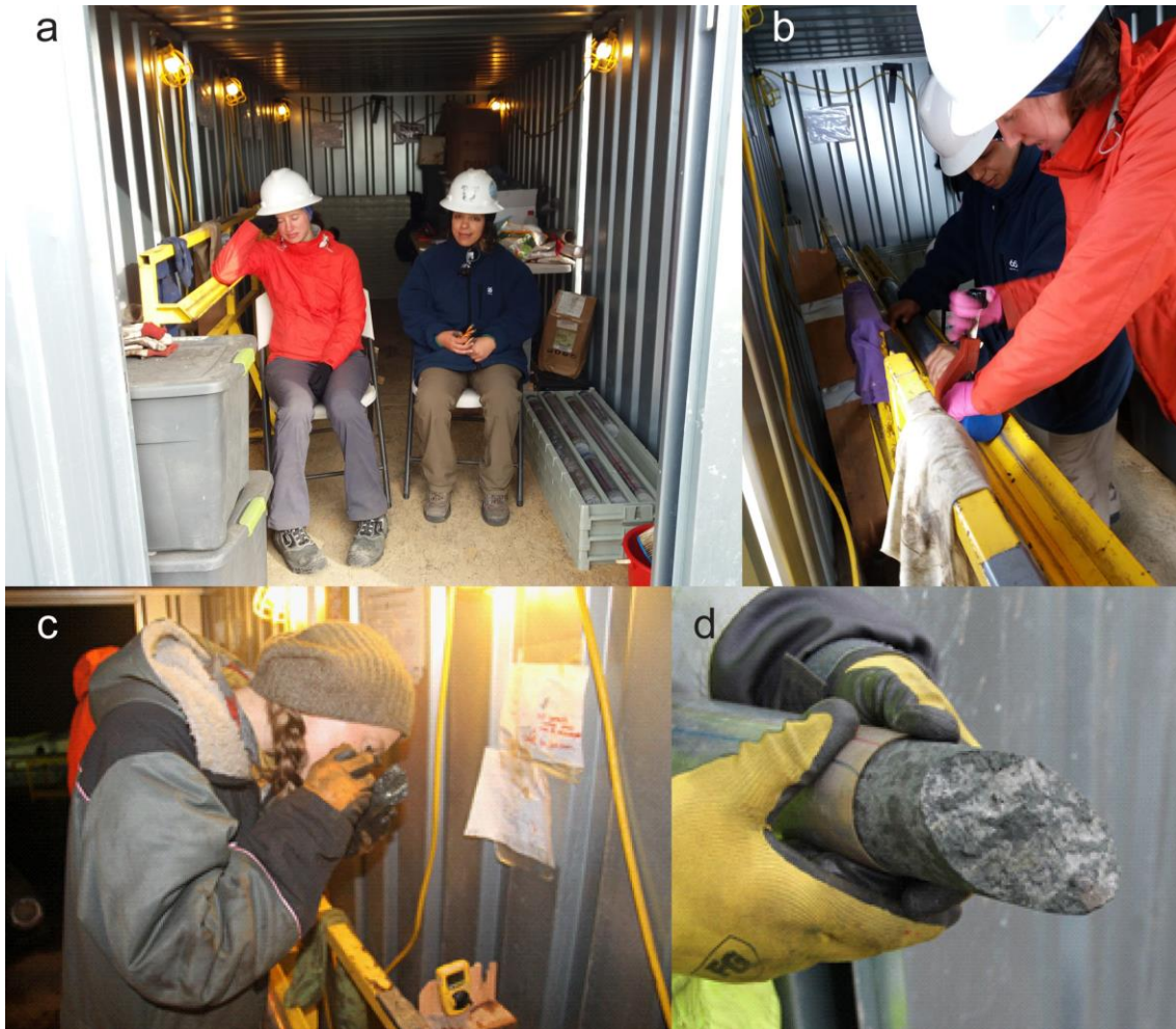
Figure 39. Photographs from the core shed at the drill site. a) Barbara Kleine (left) and Amel Barich (right) wait for the start of SE-02b coring, August 22, 2017. b) Core in plastic liner is cut with a pipe cutter. c) Carolyn F. Gorny observes a core fragment. d) Alteration minerals in the SE-03 core at about 200 m depth (photos: MTG, TBW).
