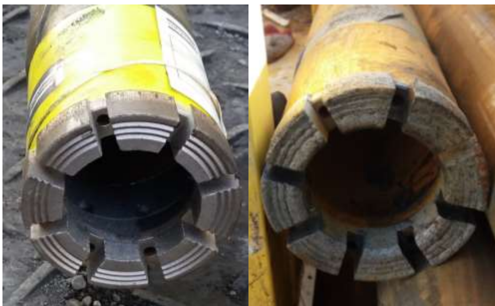
Figure 2. Core bit after 28 core runs at SE-2b after the drill string was POOH August 23 rd , 2017 (right). A image of the new core bit (left) before RIH is given for comparison (image source: TBW).
