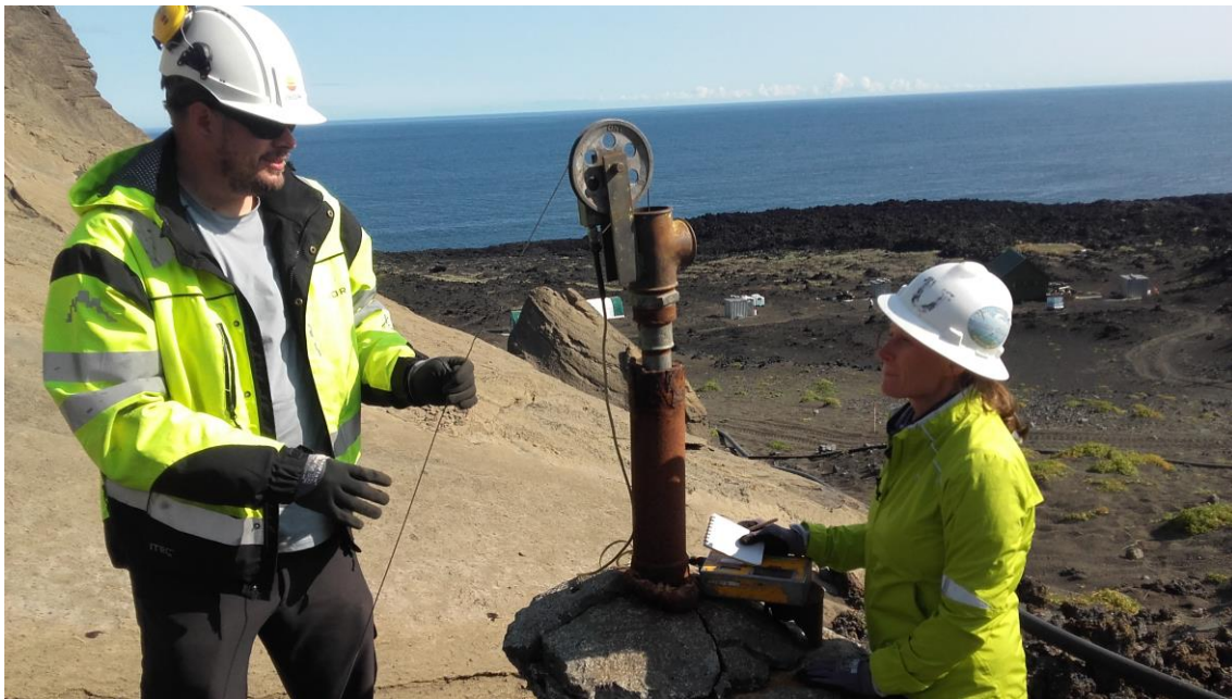
Figure 27. Photograph showing Tobias Björn Weisenberger (left) and Erica Massey (right) installing a temperature and pressure monitor string in SE-01, August 18, 2017 (photo: AB).
