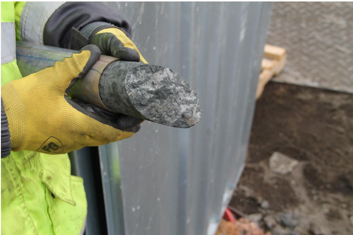
Figure 2. Alteration minerals in the core close to 200 m depth (image MTG).
