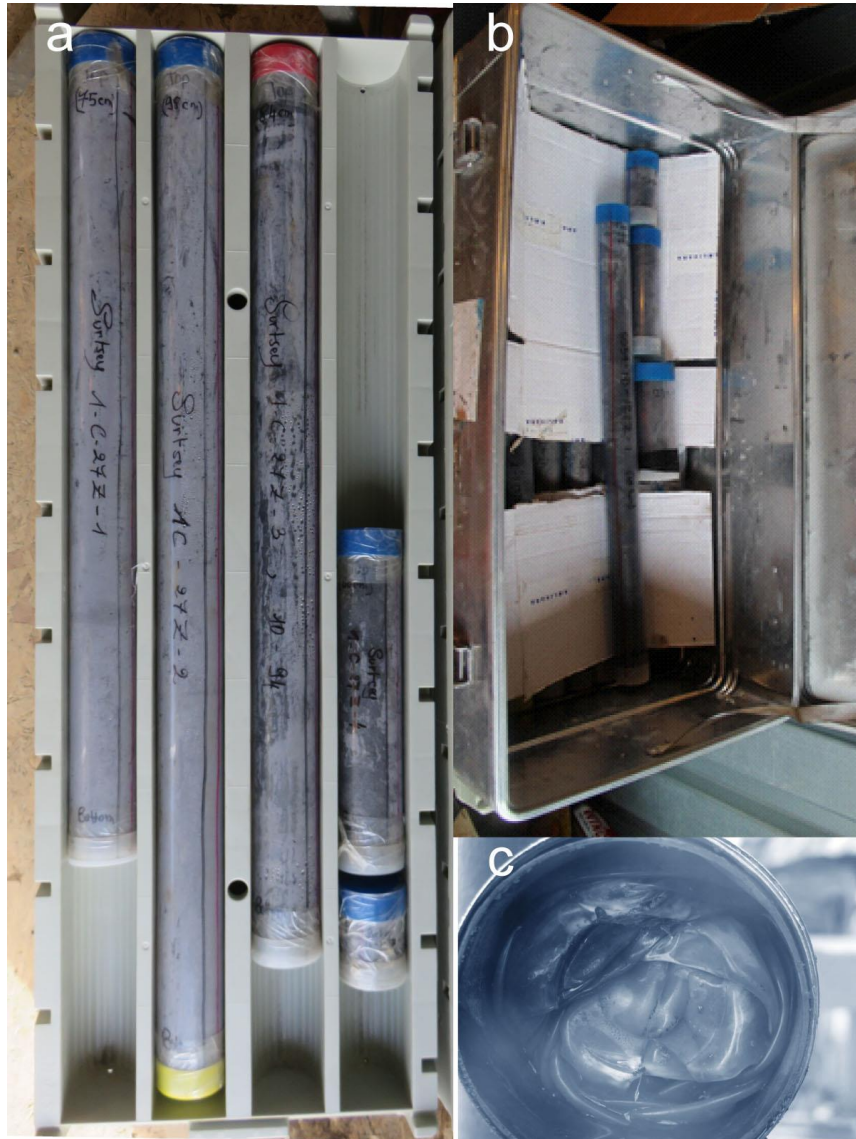
Figure 40. Cores in plastic liners on Surtsey: a) Core run 27 (5059-1-C-27-Z), borehole SE-02b, cut into four sections, and placed in portrait format in the core tray. Microbiological and geochemical samples have been taken from the top of section 3, indicated by the yellow cap at the top of section 2 and the red cap at the bottom of section 3. b) Temporary storage of SE-03 core, awaiting additional core tray delivery. c) Deformed plastic liner in the coring tube (photos: AB, MTG, TBW).
