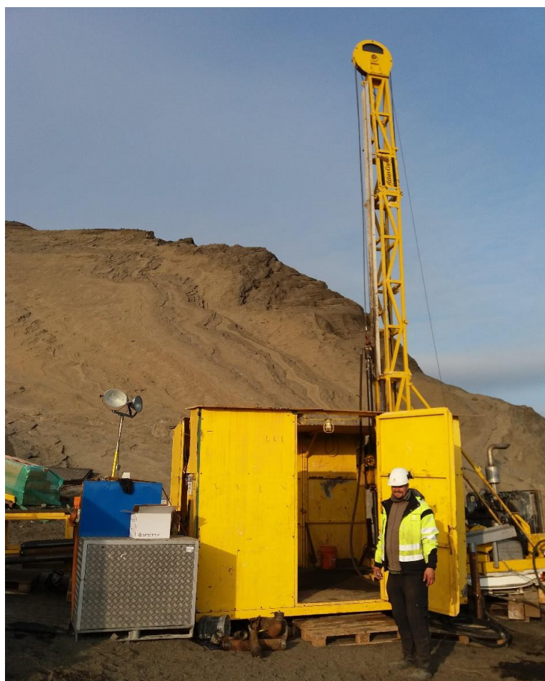
Figure 13. Photograph of the CS1000 drill rig on Surtsey (photo source: Amel Barich (AB)).
