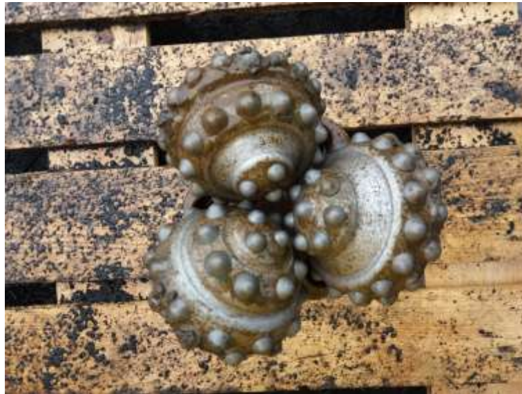
Figure 3. Tricone rotary drill bit used for drilling the pilot hole for SE-3 (image TBW).
