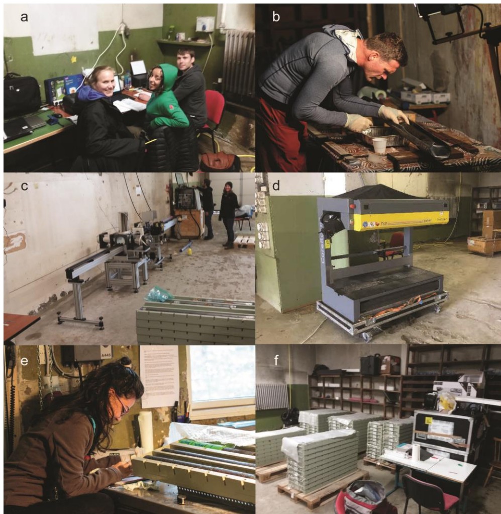
Figure 45. Photographs from the core processing laboratory on Heimaey. a) Solveig Onstad, Amel Barich, and Simon Prause work on the Digital Information System (DIS). b) Steffen Leth Jørgensen washes a section of Surtsey drill core. c) Andreas Türke and Erica Massey operate the MSCL scanner. d) DMT core scanner. e) Carla Grimaldi describes sections of Surtsey drill core. f) Core boxes ready for transport to the archive at Icelandic Institute for Natural History in Gardabaer (photos: AT, Cedric Hamelin (CH), TBW).
