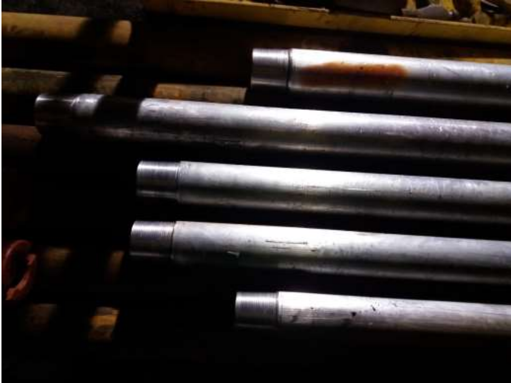
Figure 4. Picture showing the different length of the pipe for the Al casing for SE-2b (image TBW).
