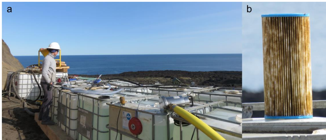
Figure 15. Photograph showing seawater storage at the drill site. a) Barbara Kleine, managing the water sterilization system. b) Used water filter (photo: AB).
