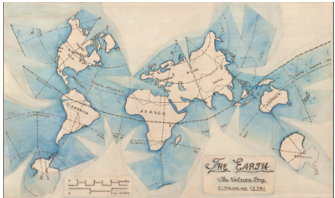
On pages 8 to 11 there was a discussion of the problems associated by presenting the globe on a flat map, leading to distortion of shapes and sizes. This map, by the author, is composed of 60 triangle polyhedron, and presents shapes and sizes almost as they actually are on the globe itself.
