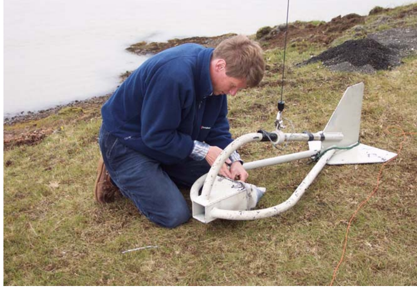
Figure 3: Bedload sampling at the cableway at Krókur, Þjórsá.
