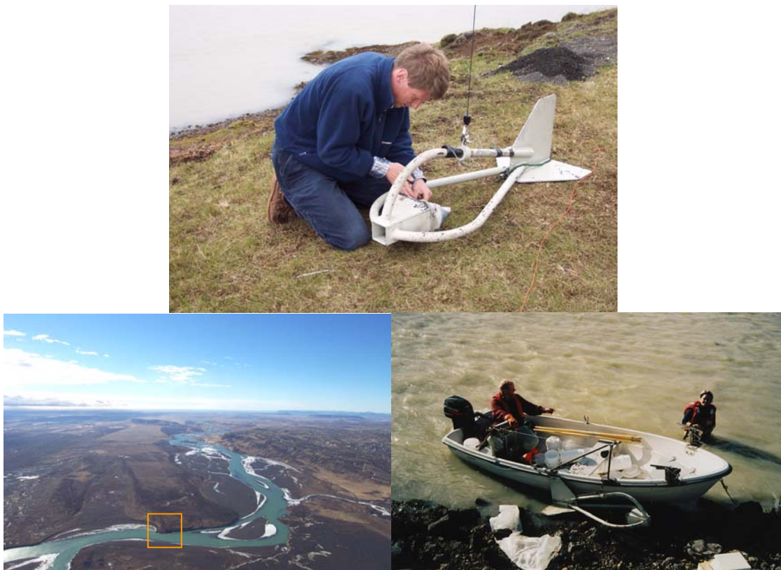
Figure 3: Top: Bedload sampling at the cableway at Krókur, Þjórsá (Photo: Arndís Ólafsdóttir). Bottom left: The location of bedload sampling at Sandártunga, Þjórsá (Photo: Jörunn Harðardóttir). Bottom right: The specially equipped boat used for bedload sampling at Sandártunga, Þjórsá, here used at Sóleyjarhöfði, Þjórsá (Photo: Steen Henriksen).
