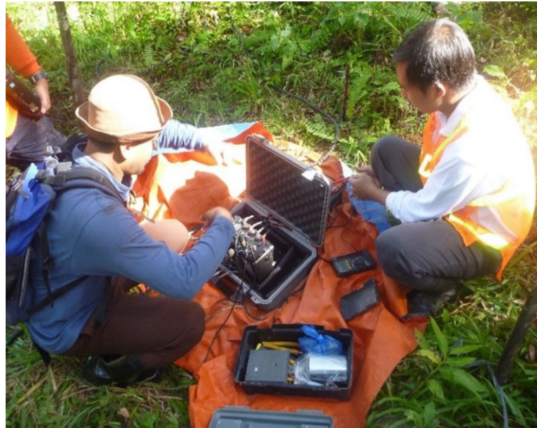
FIGURE 6: MT data acquisition in Mainit geothermal area using Phoenix MT instruments (09 July, 2012)
