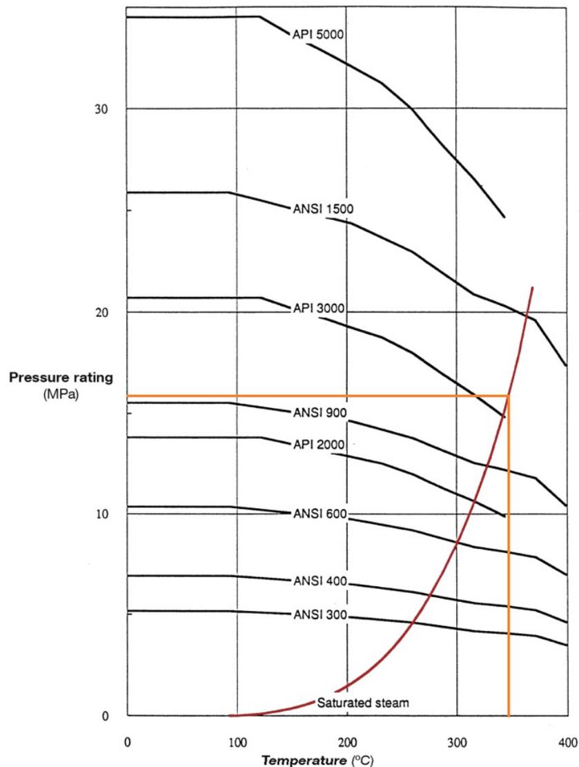
FIGURE 10: Wellhead working pressure de-rating for flanges and valves; the yellow line represents the maximum wellhead conditions (African Union Standard, 2016)
