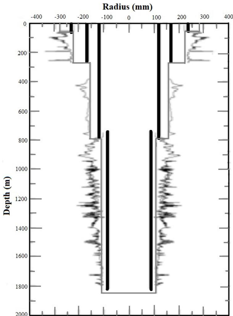
FIGURE 2: Schematic picture of a geothermal well, showing casing (bold lines) and drill bit sizes (soft straight lines) and caliper logs (Steingrímsson, 2011)
