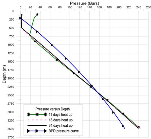
FIGURE 6: OW-736A pressure profiles and adjusted BP pressure curve
