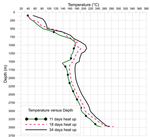
FIGURE 5: OW-736A temperature depth profiles
