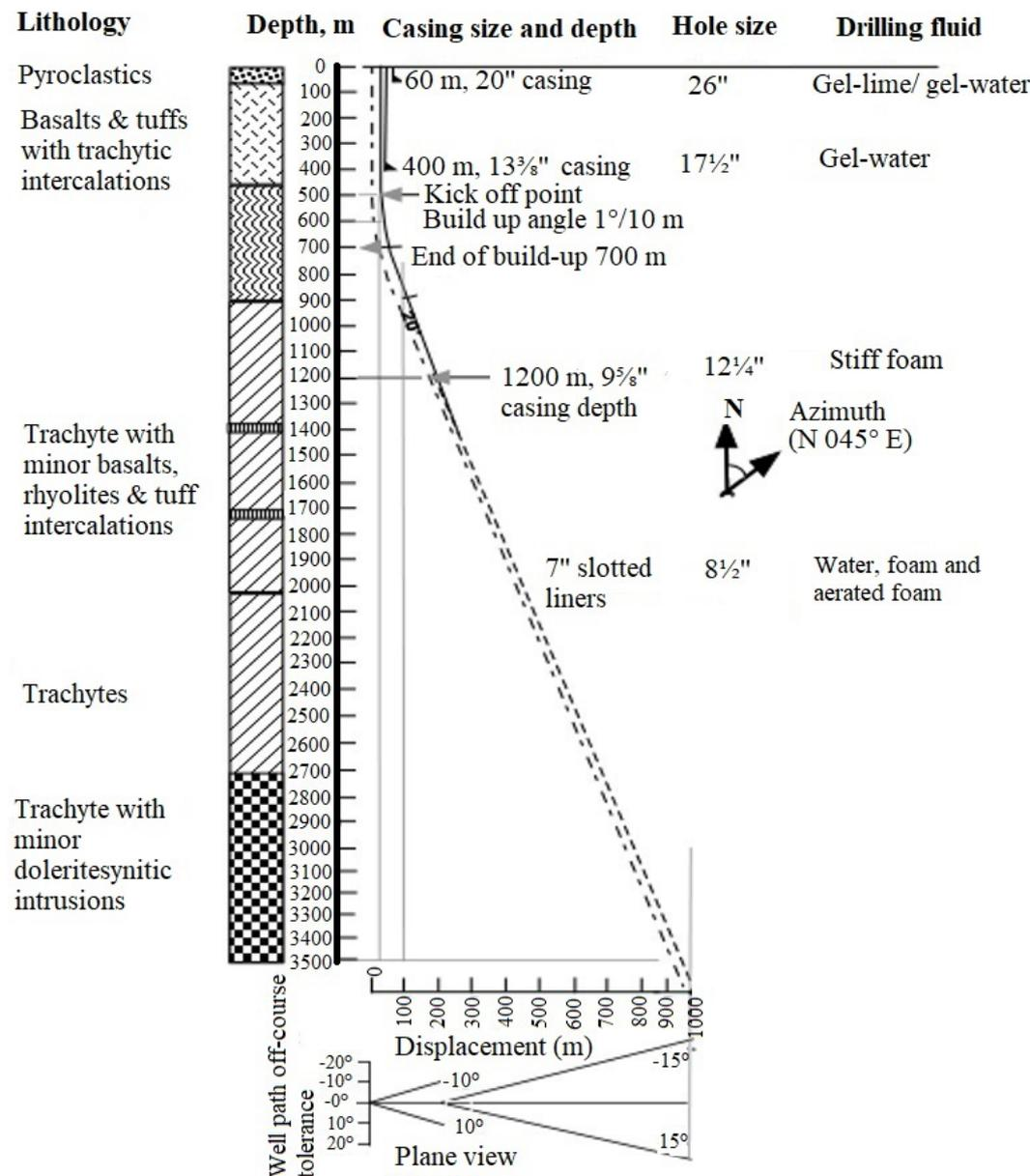
FIGURE 1: Well OW-736A design and geological cross-section (KenGen, 2014)
