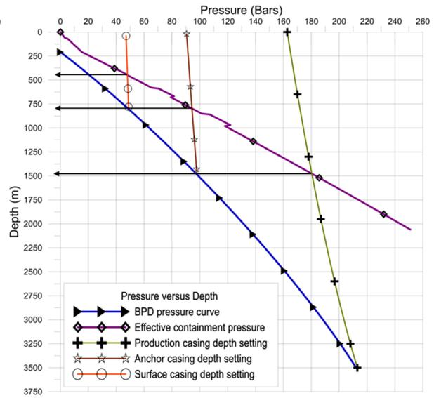
FIGURE 9: Redesigned well OW 736A minimum casing depth setting assuming pressure from static steam column
