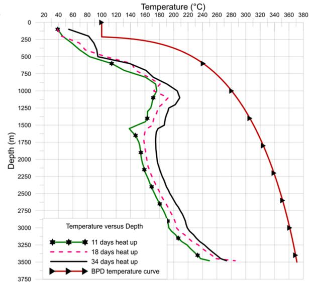
FIGURE 7: OW-736A temperature profiles and adjusted BP temperature curve
