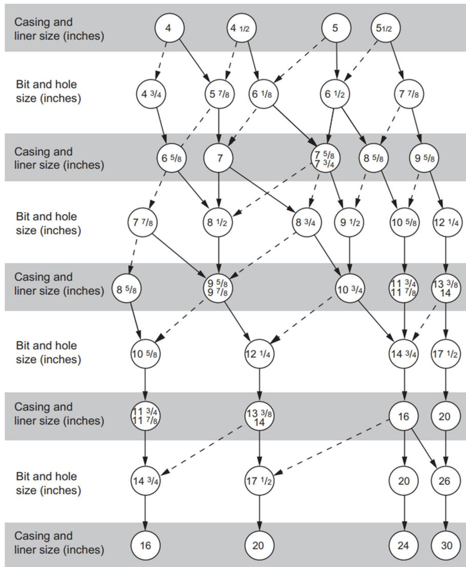
FIGURE 3: Casing sizes and hole configurations (Heriot, Watt University, 2010)
