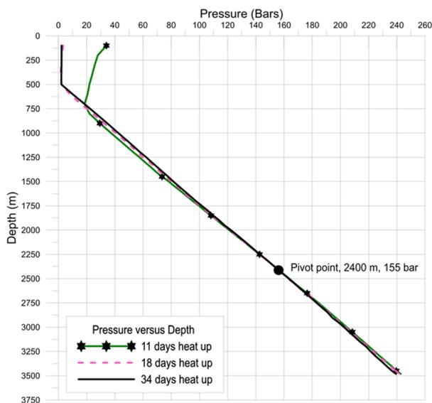
FIGURE 4: OW-736A pressure depth profiles
