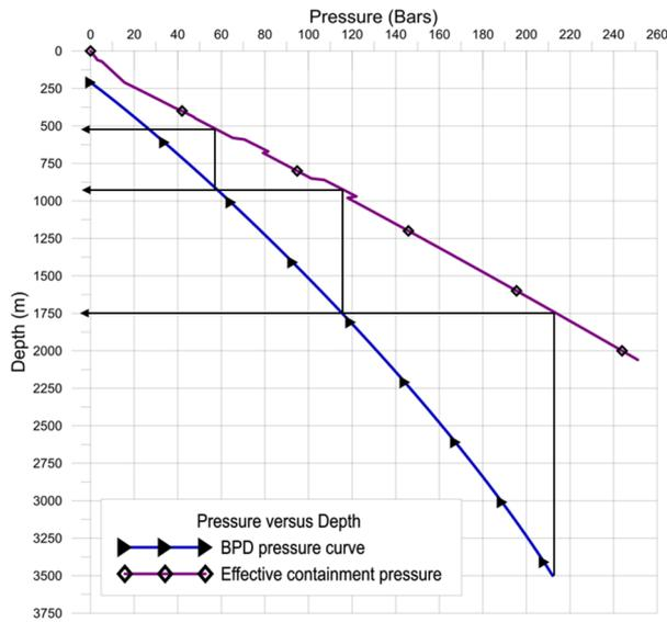
FIGURE 8: Redesigned well OW 736A minimum casing depth setting assuming constant pressure column
