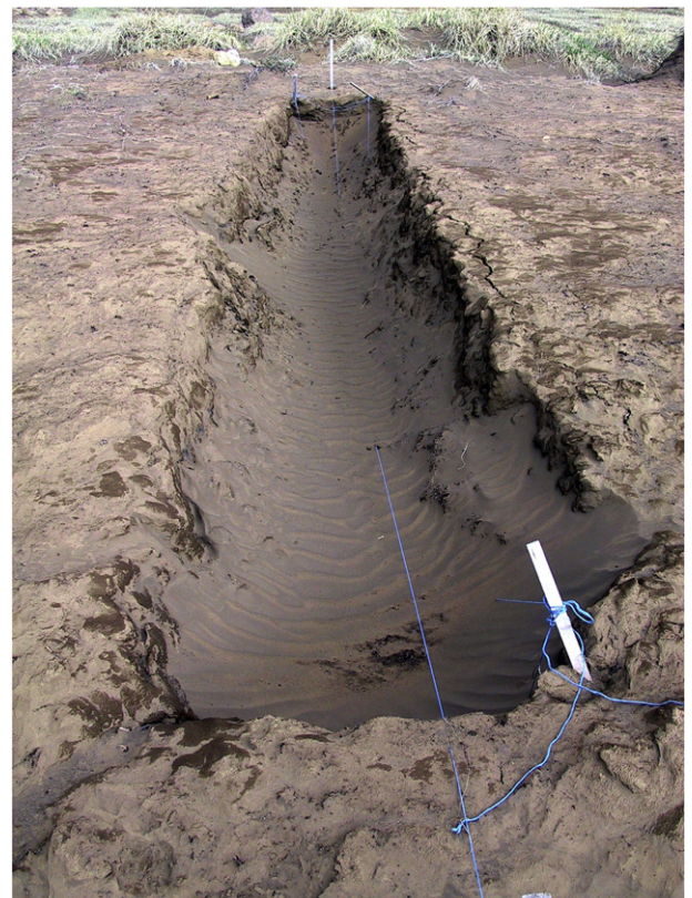
Fig. 7. Sediment ditch at Holsfjöll after the first year. It was originally 1 m deep and it filled up in 2 yrs, indicating >1000 \text{ kg m}^{-1} sediment transport during that time.
