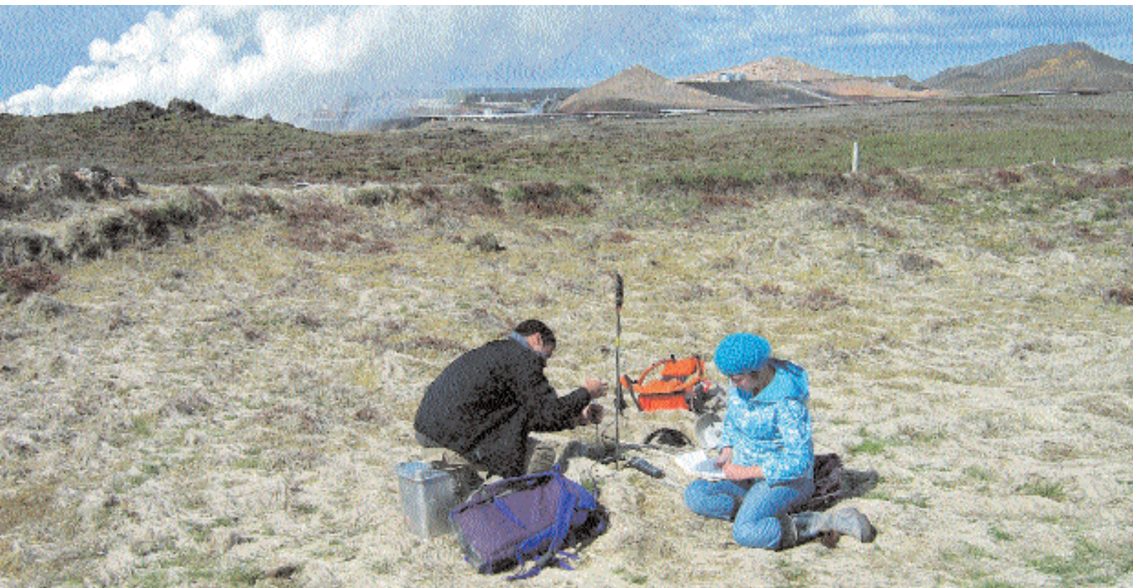
▲ Measuring natural CO 2 emissions in the Reykjanes geothermal area. Photo Bjarni Reyr Kristjánsson.
