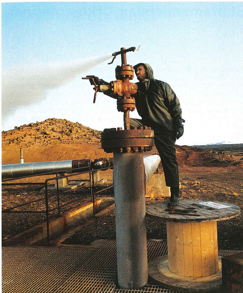
Preparation for sampling from well 9 in the Reykjanes high-temperature geothermal area, in November 1992. Photo. Ragnhildur Sigurðardóttir.
