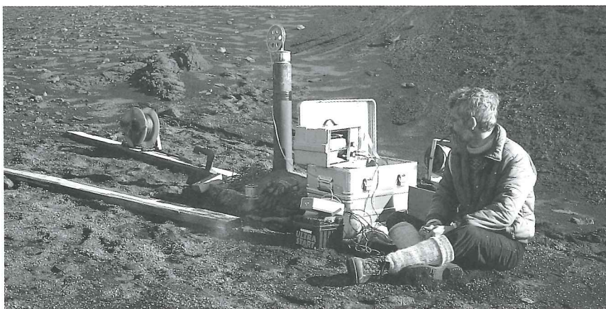
Mæling borholu í Surtsey (ljósm./photo, Magnús Ólafsson) Logging of an exploratory well on the island of Surtsey.
